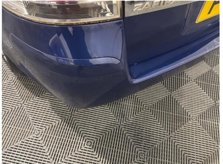
10: Bumper Rear Scratched Over 100mm Thru Paint
