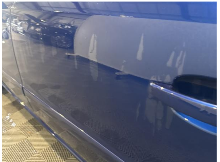
6: Door nsr Dented 2 Or Less UpTo 10mm
