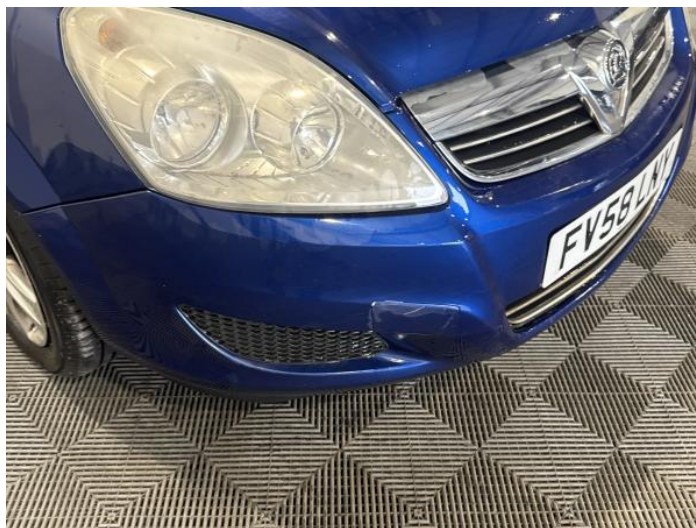
2: Bumper Front Scratched Over 100mm Thru Paint
