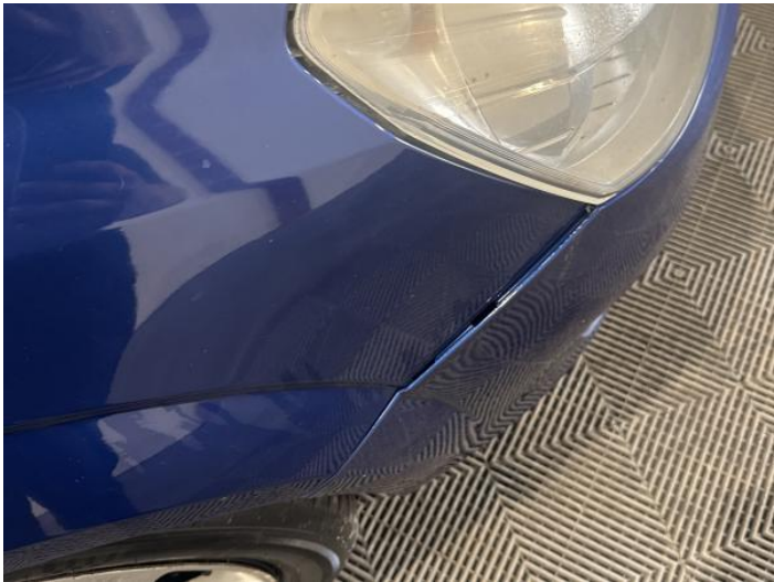
18: Wing osf Dented With Paint Damage
