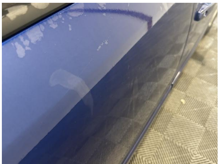
14: Door osf Scratched Over 25mm Thru Paint
