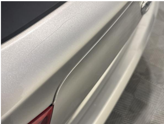
11: Boot Lid Scratched Over 25mm Thru Paint
