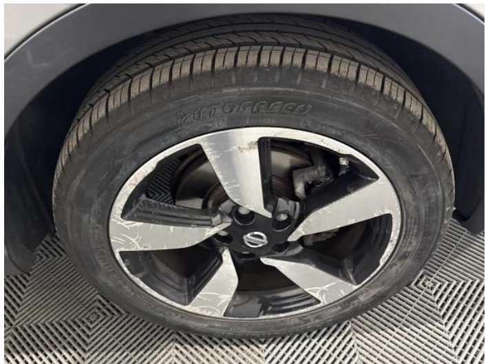
18: Wheel osf Scratched Over 50mm
