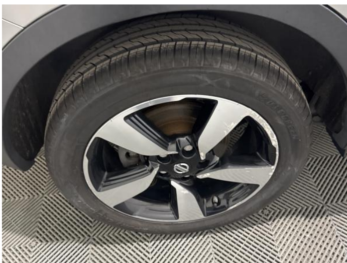
13: Wheel osr Scratched Over 50mm
