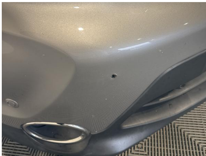
2: Bumper Front Hole UpTo 25mm
