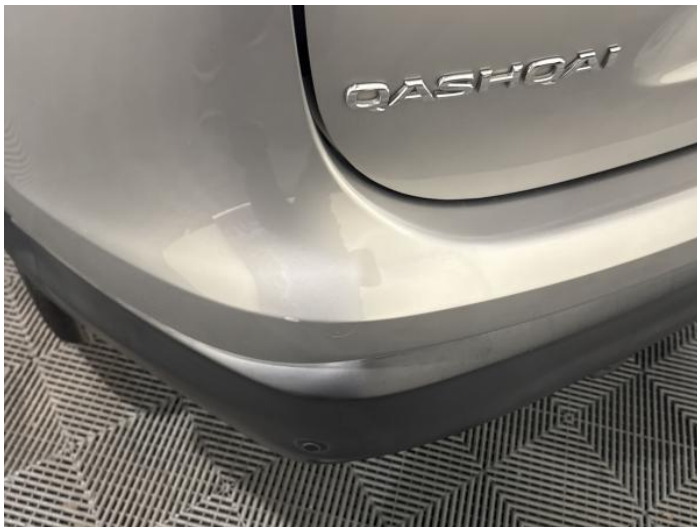
9: Bumper Rear Scratched 25 to 100mm Thru Paint
