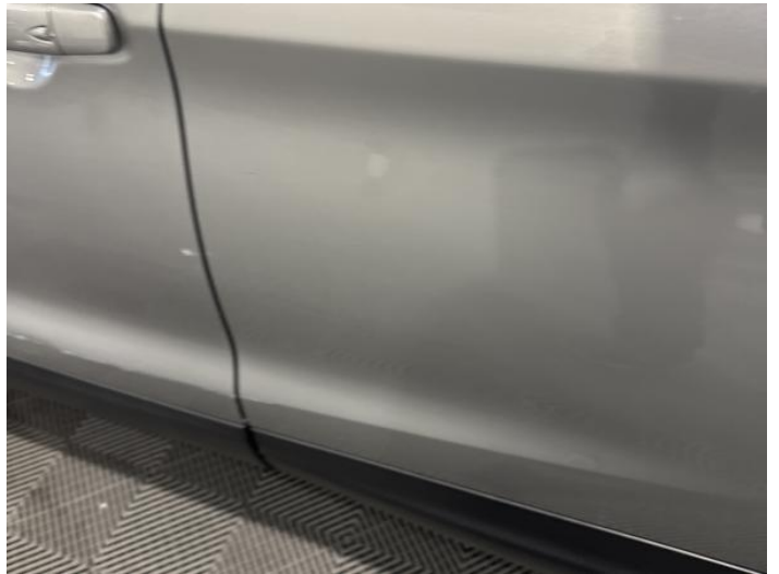
6: Door nsr Scratched Over 25mm Thru Paint
