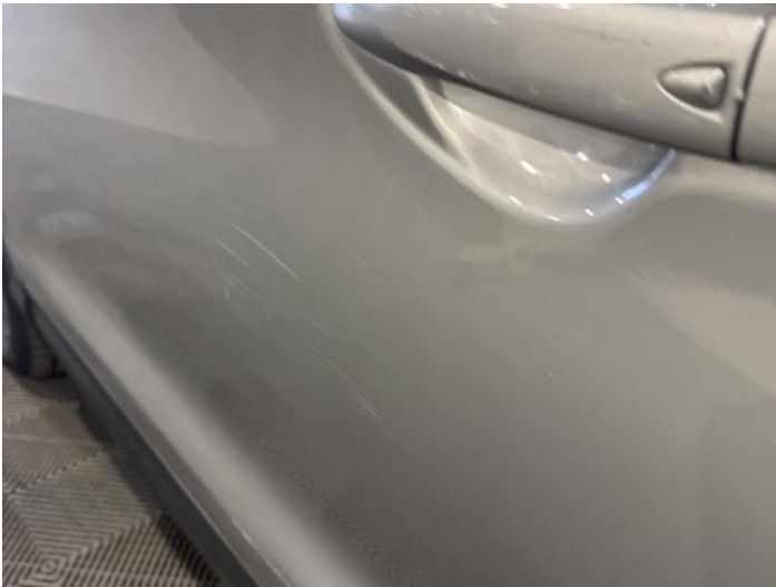
5: Door nsf Scratched Over 25mm Thru Paint
