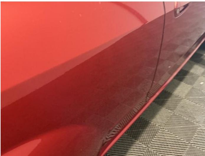
11: Qtr Panel osr Dented 2 Or Less UpTo 10mm
