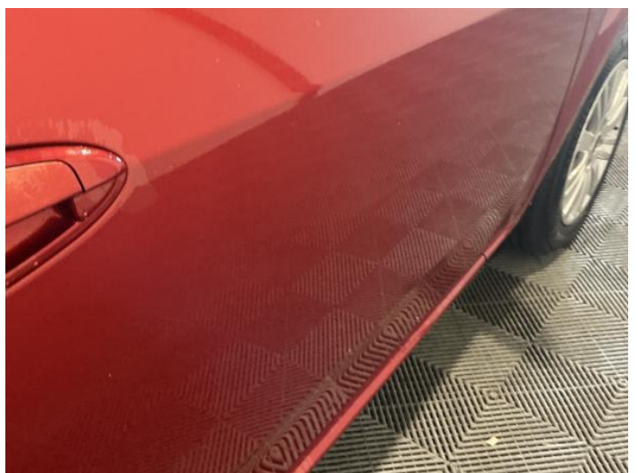
14: Door osf Dented Over 2 UpTo 10mm
