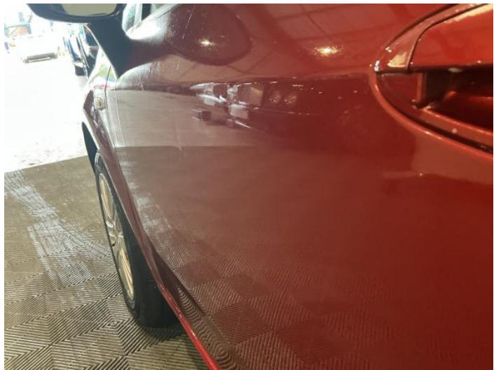
6: Door nsf Dented Over 30mm
