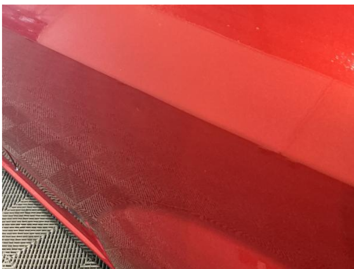
7: Qtr Panel nsr Dented Over 30mm
