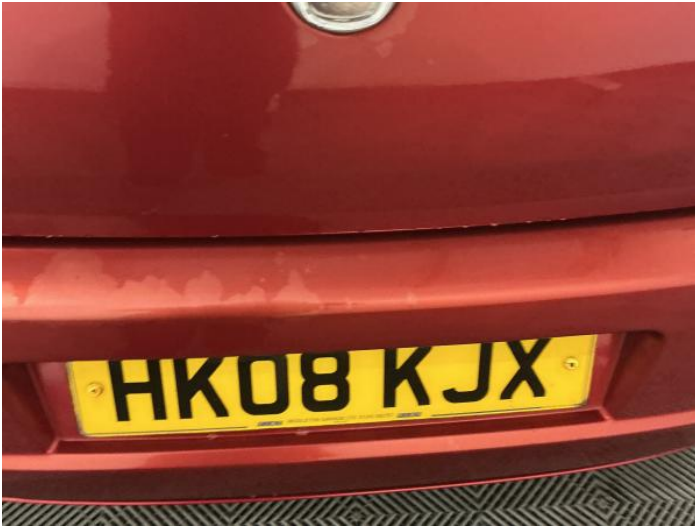
9: Bumper Rear Poor Previous Repair Paint Flake
