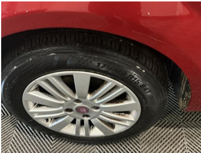
5: Wheel nsf Scratched Over 50mm
