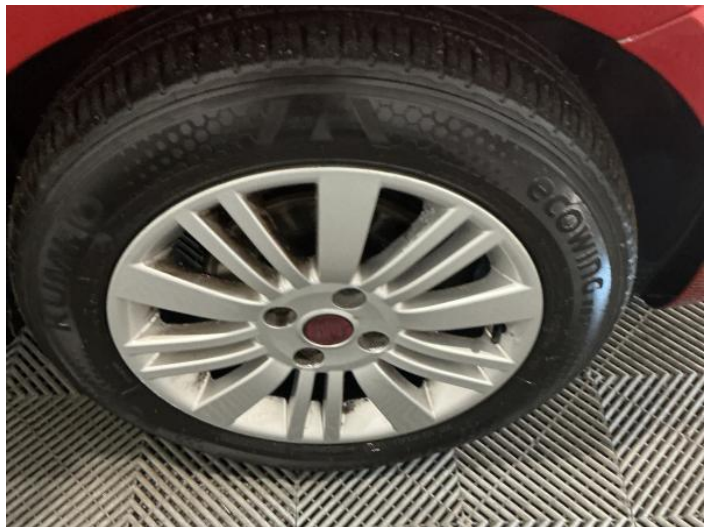
16: Wheel osf Scratched Over 50mm
