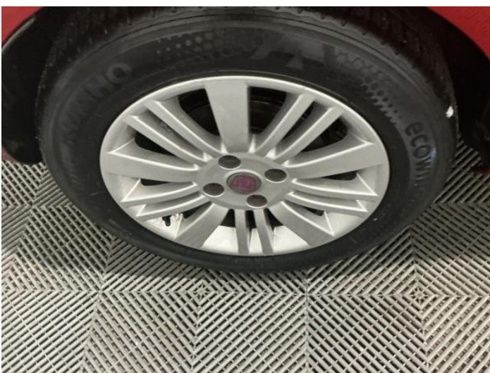
13: Wheel osr Scratched Over 50mm
