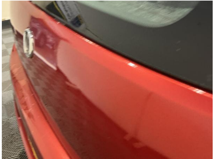
10: Boot Lid Dented Between 10mm + 30mm
