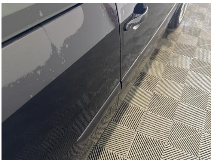
17: Qtr Panel osr Dented Between 10mm + 30mm
