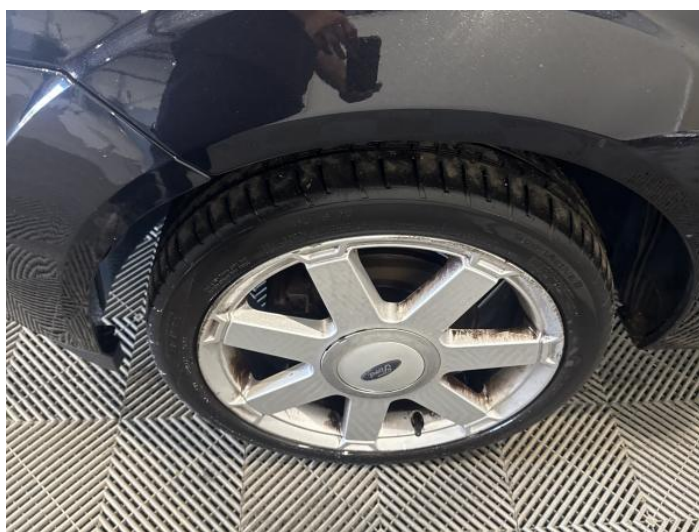
6: Wheel nsf Scratched Over 50mm
