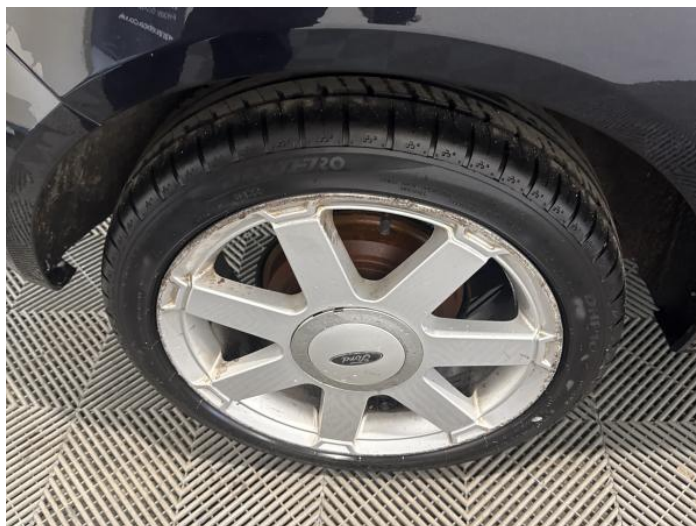
16: Wheel osr Scratched Over 50mm
