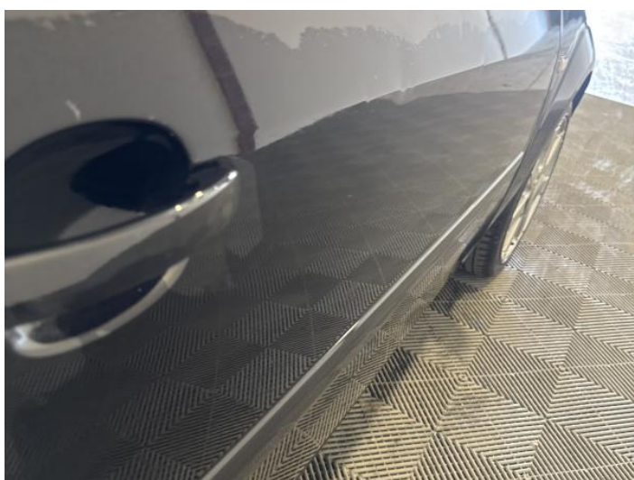
19: Door osf Dented Over 2 UpTo 10mm
