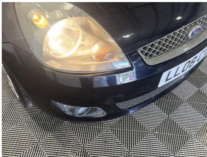
4: Bumper Front Scratched 25 to 100mm Thru Paint
