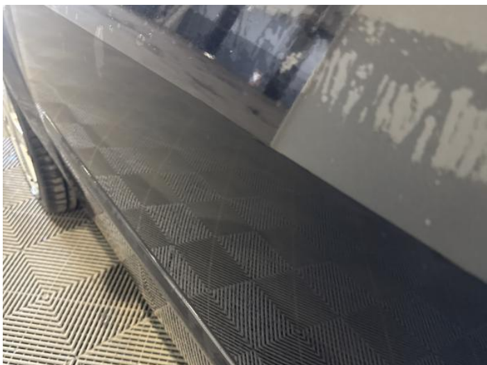
9: Door nsf Dented Over 2 UpTo 10mm
