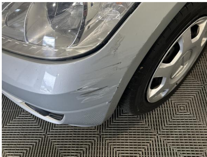
2: Bumper Front Scratched 25 to 100mm Thru Paint
