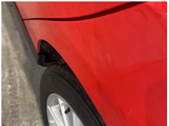
6: Qtr Panel nsr Dented Over 2 UpTo 10mm
