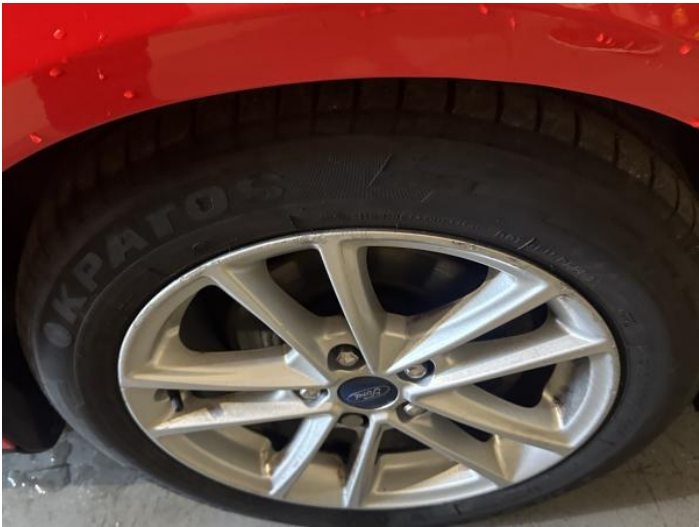
17: Wheel osf Scratched Over 50mm
