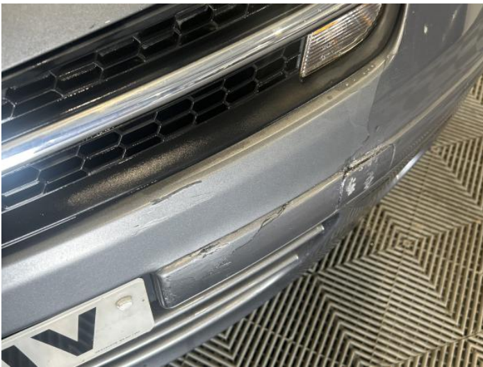
17: Bumper Front Poor Previous Repair Paint Flake
