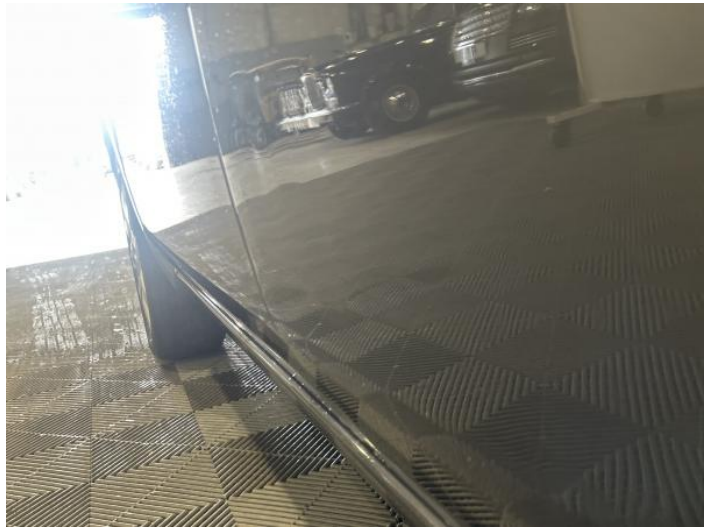
12: Door nsr Dented Over 30mm
