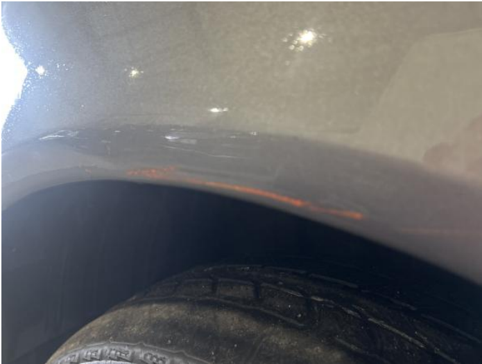
15: Wing nsf Poor Previous Repair Poor Paint
