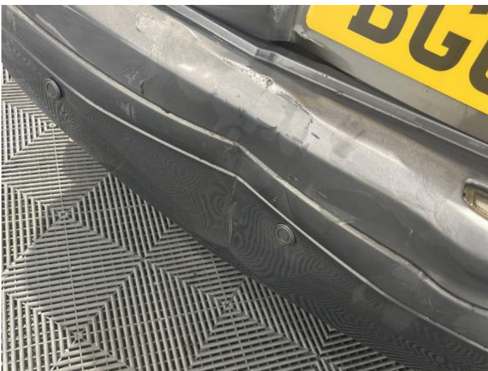
7: Bumper Rear Dented Over 30% Of Panel
