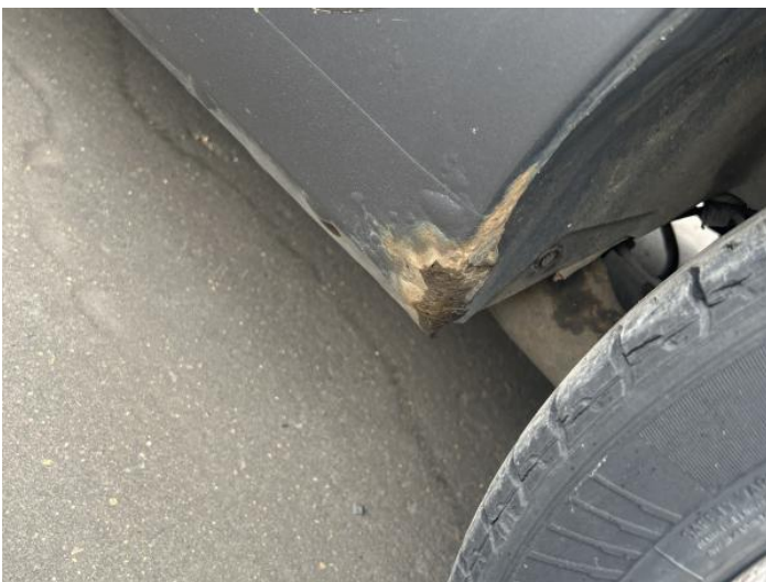
19: Sill ns Rusted Over 5mm
