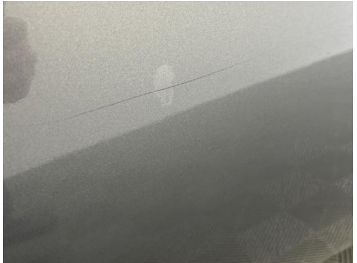
4: Door osr Scratched Over 25mm Thru Paint
