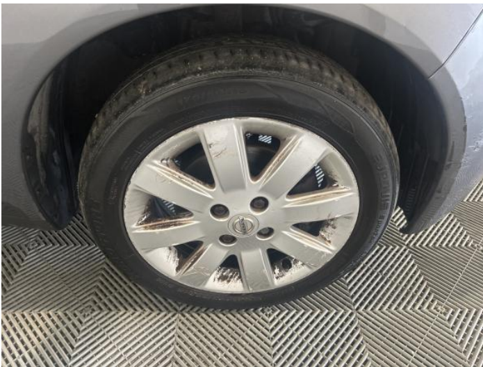
1: Wheel osf Scratched Over 50mm
