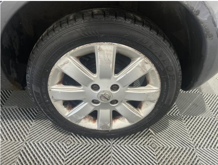
11: Wheel nsr Scratched Over 50mm
