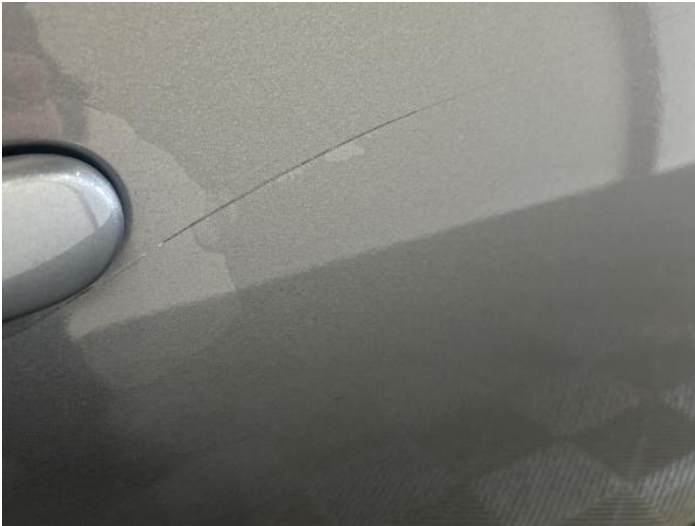
3: Door osf Scratched Over 25mm Thru Paint
