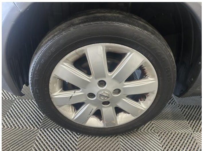
14: Wheel nsf Scratched Over 50mm
