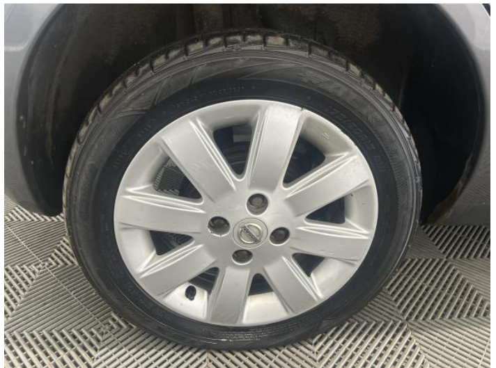
6: Wheel osr Scratched Up To 50mm
