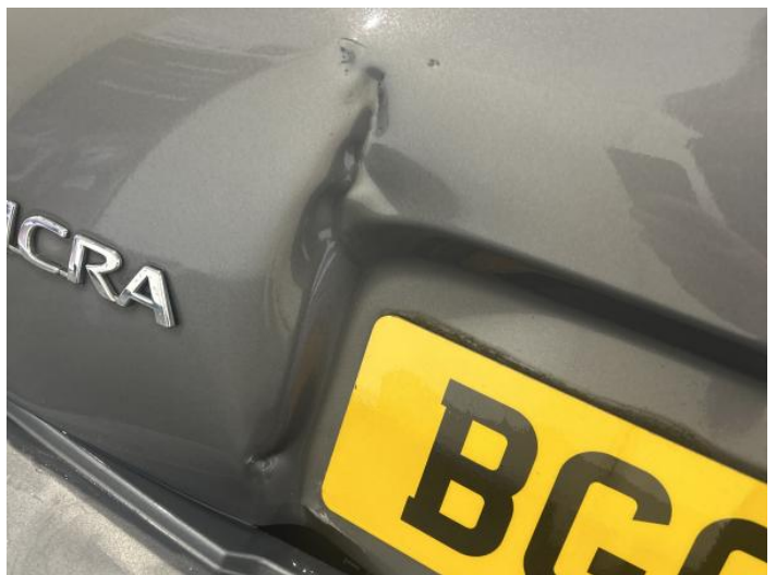
8: Tailgate Dented Over 30% Of Panel
