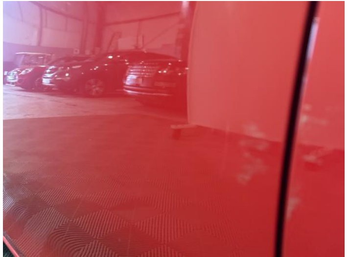
16: Door nsf Scratched Over 25mm Not Thru Paint
