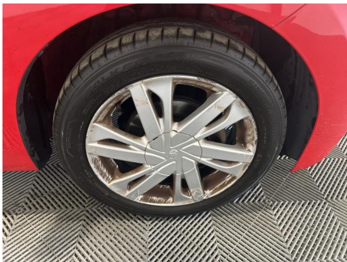
1: Wheel osf Scratched Over 50mm
