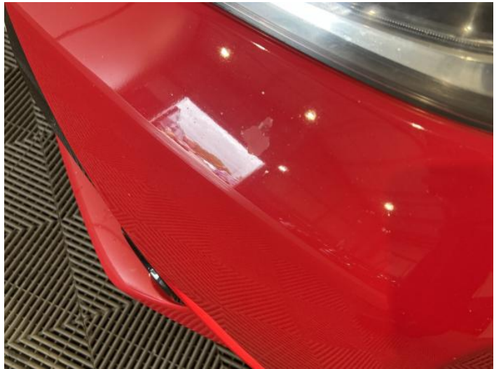
18: Bumper Front Poor Previous Repair Paint Flake
