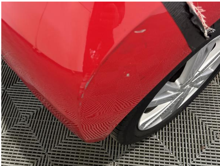
9: Bumper Rear Scratched 25 to 100mm Thru Paint
