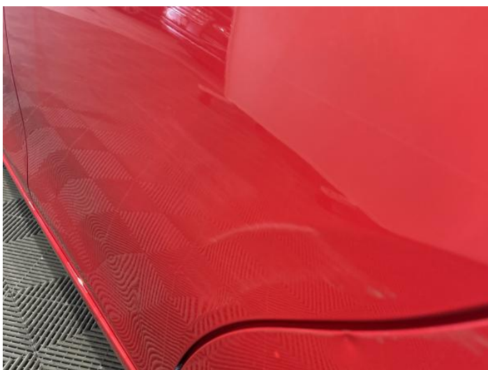
13: Door nsr Dented With Paint Damage
