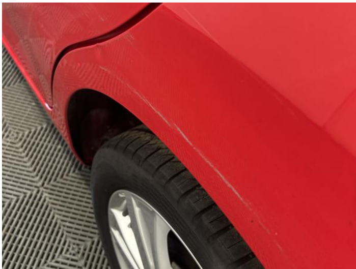
11: Qtr Panel nsr Dented With Paint Damage
