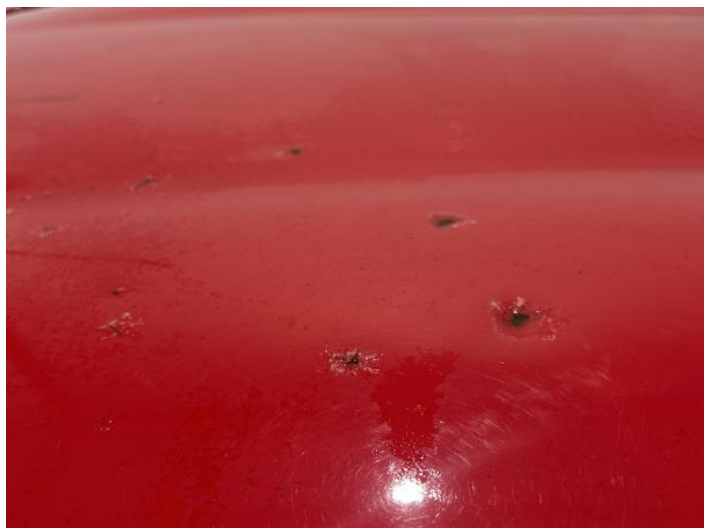
20: Roof Dented With Paint Damage
