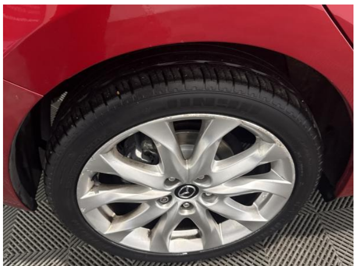
14: Wheel osr Scratched Over 50mm
