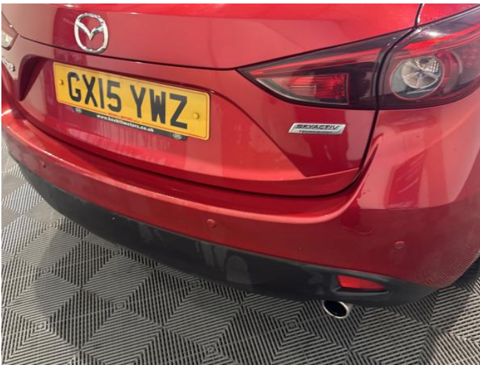
11: Bumper Rear Scratched 25 to 100mm Thru Paint
