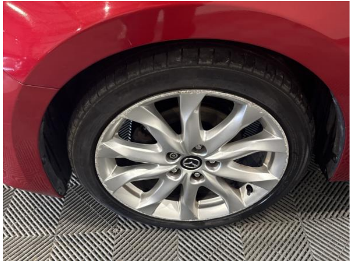
4: Wheel nsf Scratched Over 50mm
