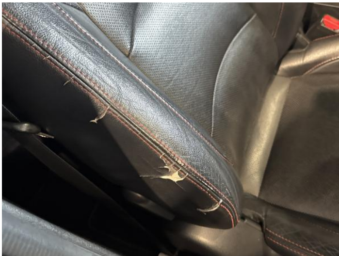
1: Seat Back Cover osf Torn Over 3mm
