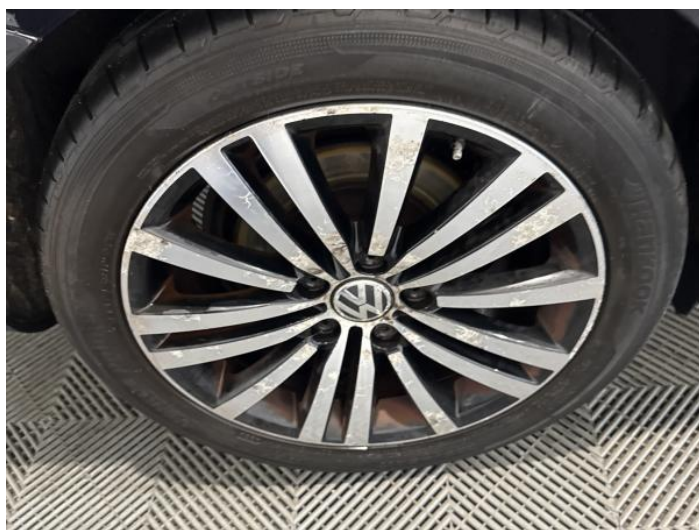
20: Wheel osr Scratched Over 50mm
