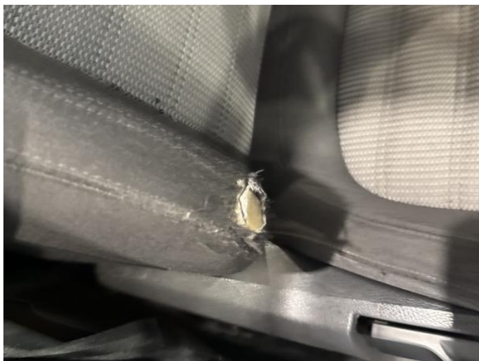
1: Seat Back Cover osf Torn Over 3mm
