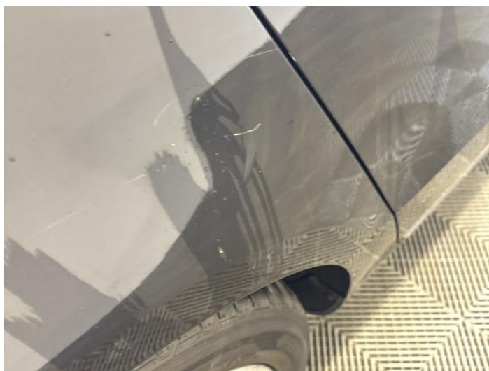
18: Qtr Panel osr Scratched UpTo 25mm Thru Paint
