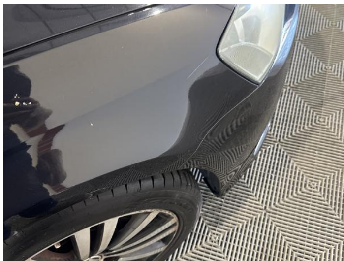
24: Wing osf Scratched Over 25mm Thru Paint
