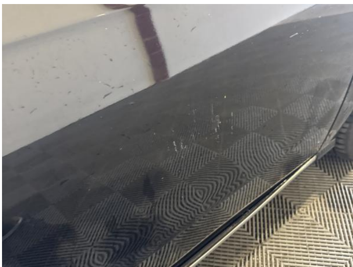
23: Door osf Chipped Multiple Chips
