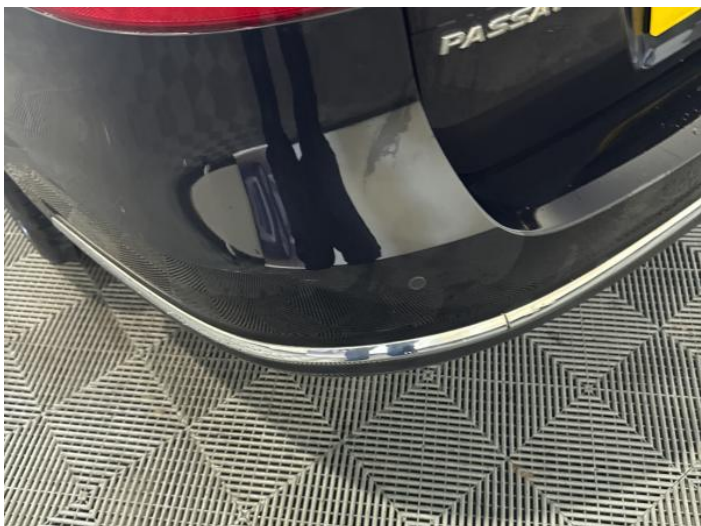
15: Bumper Rear Scratched 25 to 100mm Thru Paint
