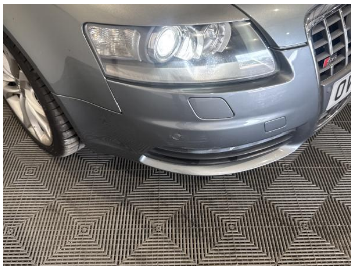
2: Bumper Front Scratched 25 to 100mm Thru Paint
