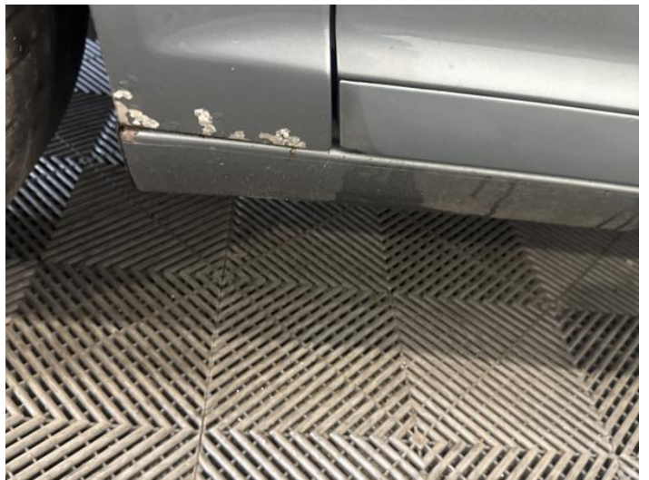
6: Sill ns Scratched UpTo 25mm Thru Paint
