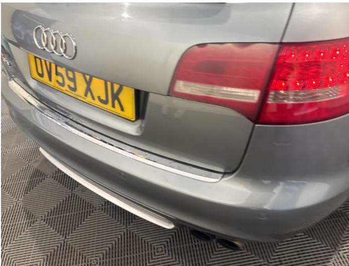
11: Bumper Rear Chipped Multiple Chips
