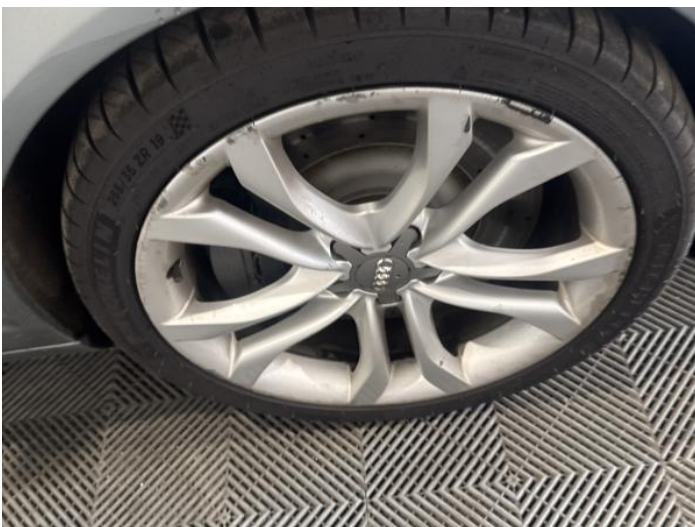
19: Wheel osf Scratched Over 50mm
