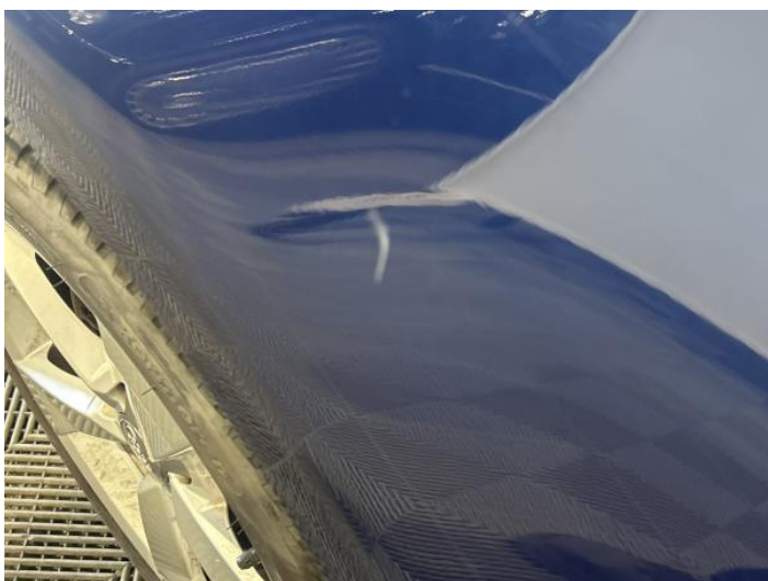
7: Wing nsf Scratched UpTo 25mm Thru Paint
