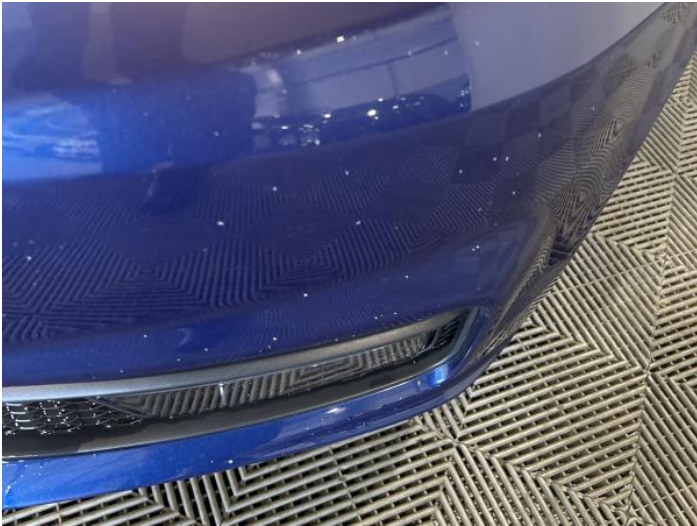
9: Bumper Front Chipped Multiple Chips
