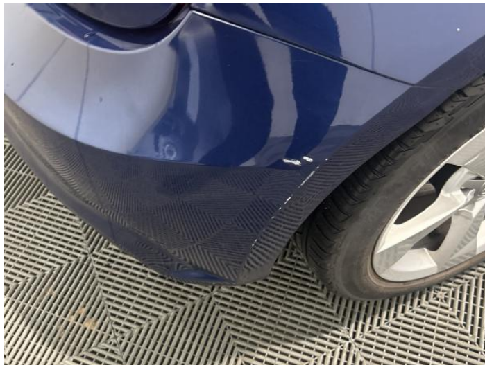
4: Bumper Rear Scratched 25 to 100mm Thru Paint
