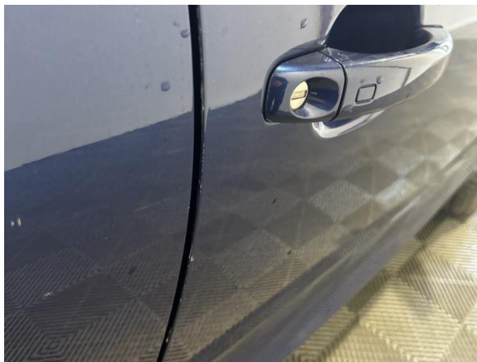
2: Door osf Chipped Edge Chip
