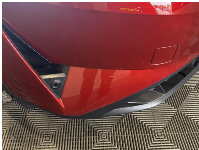
2: Bumper Front Scratched 25 to 100mm Thru Paint
