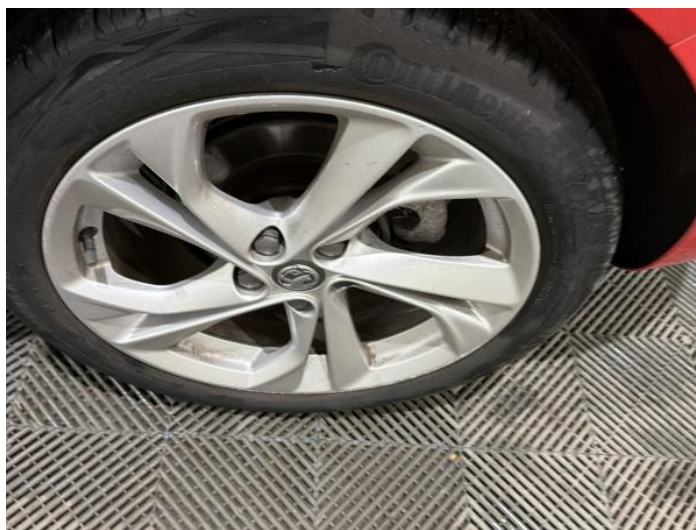
12: Wheel nsr Scratched Up To 50mm
