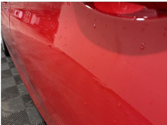
9: Door nsr Dented 2 Or Less UpTo 10mm
