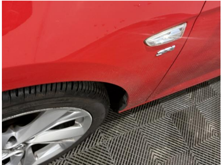
4: Wing nsf Dented Over 2 UpTo 10mm
