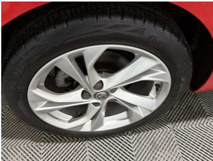
17: Wheel osr Scratched Up To 50mm
