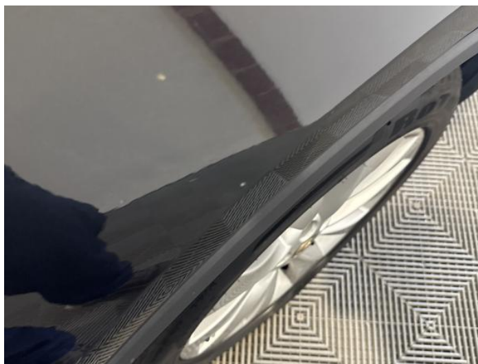
18: Wing osf Poor Previous Repair Poor Paint
