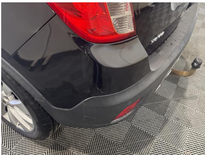
11: Bumper Rear Scratched Over 100mm Thru Paint
