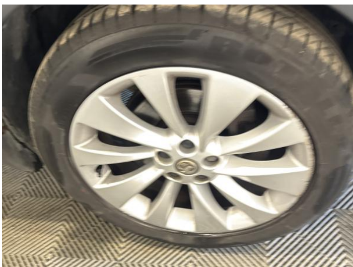
19: Wheel osf Scratched Over 50mm
