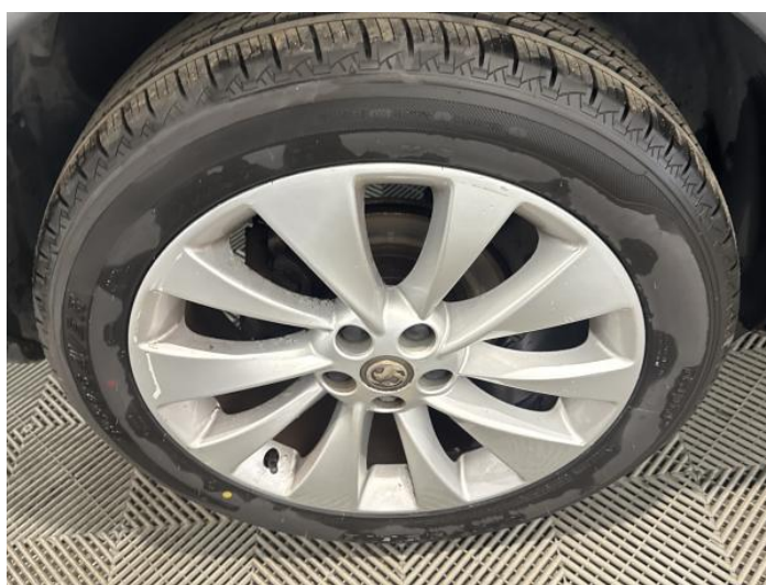
14: Wheel osr Scratched Over 50mm
