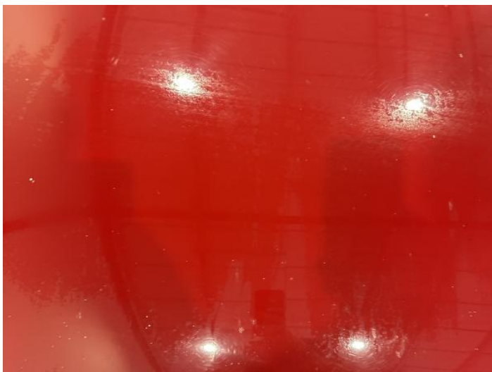
1: Bonnet Chipped Multiple Chips
