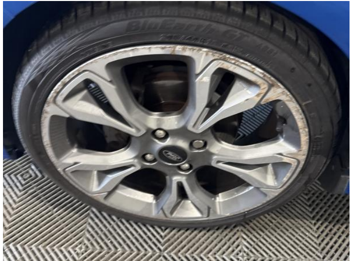
4: Wheel nsf Scratched Over 50mm
