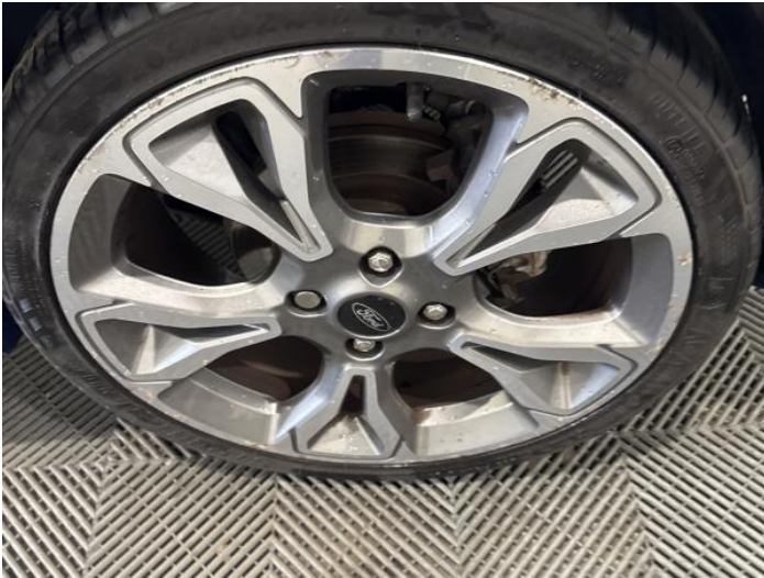
9: Wheel nsr Scratched Over 50mm
