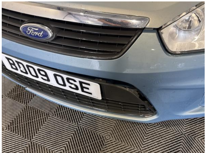
2: Bumper Front Grill Broken Replace
