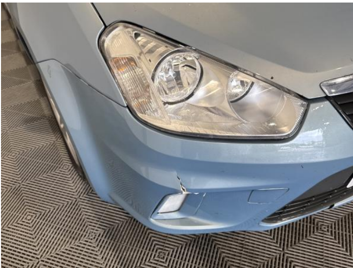
1: Bumper Front Cracked Over 25mm
