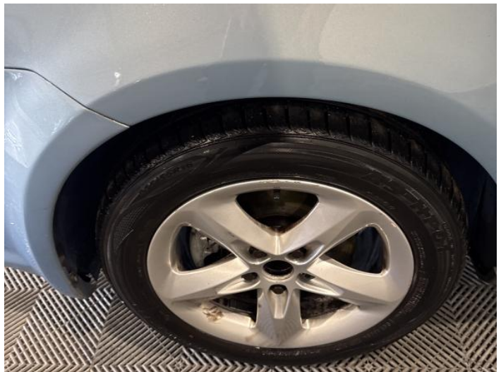
4: Wheel nsf Scratched Over 50mm
