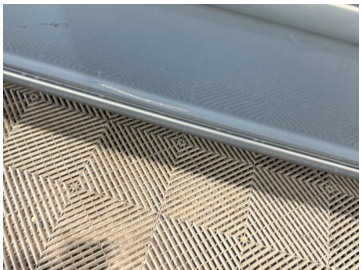
6: Door nsf Dented With Paint Damage
