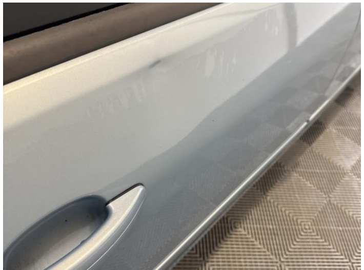
16: Door osr Dented Between 10mm + 30mm
