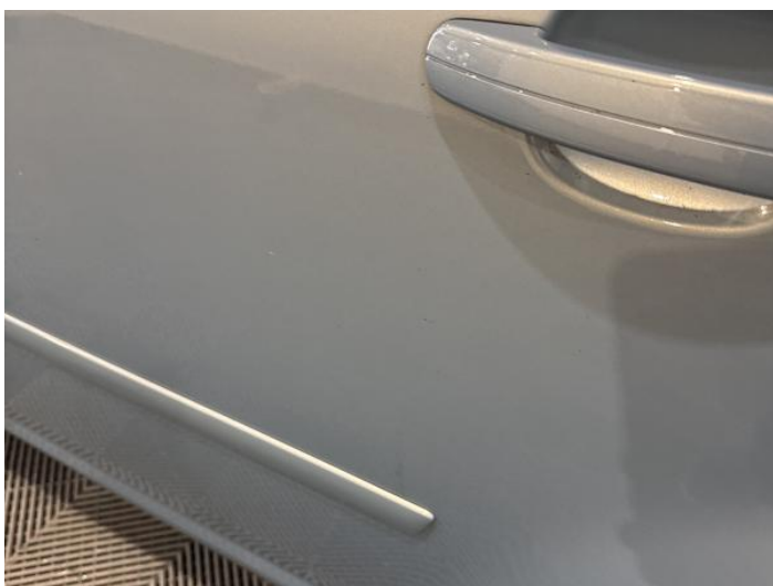
7: Door nsr Dented 2 Or Less UpTo 10mm
