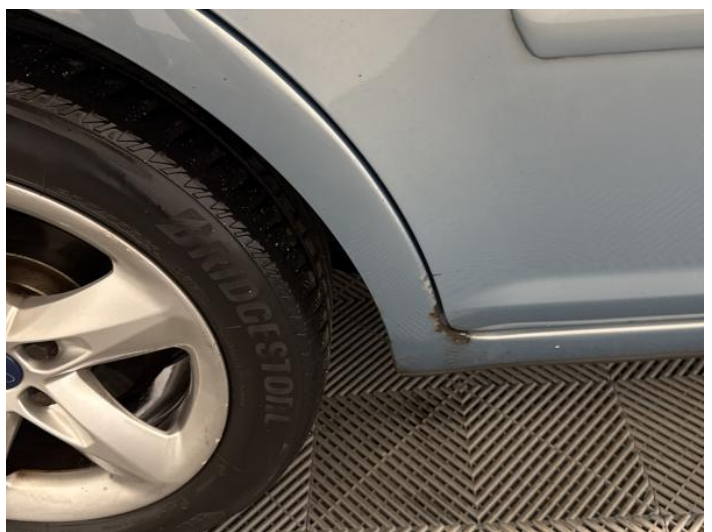
14: Qtr Panel osr Rusted Over 5mm
