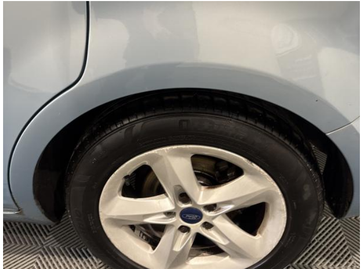
10: Wheel nsr Scratched Over 50mm
