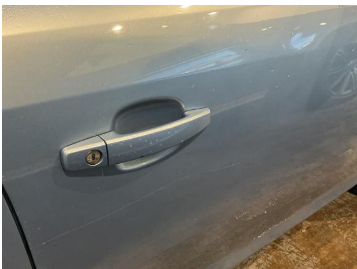
11: Door osf Scratched Over 25mm Thru Paint
