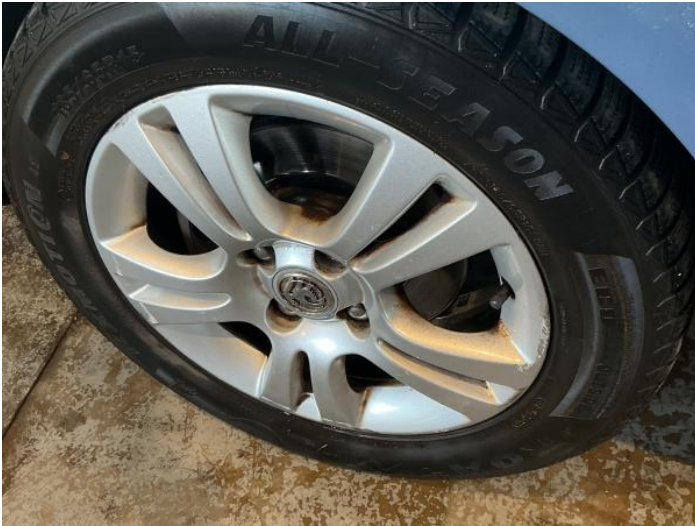
3: Wheel nsf Scratched Over 50mm
