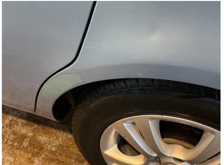
6: Qtr Panel nsr Poor Previous Repair Poor Paint
