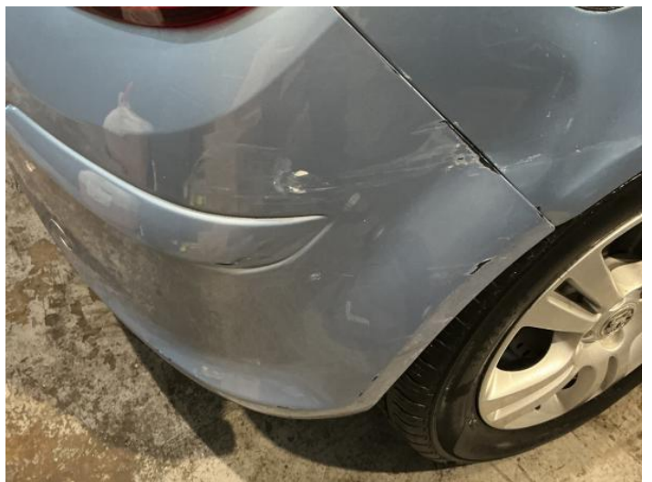
8: Bumper Rear Scratched Over 100mm Thru Paint
