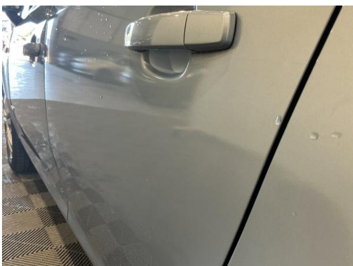
13: Door nsr Poor Previous Repair Rippled UpTo 30%
