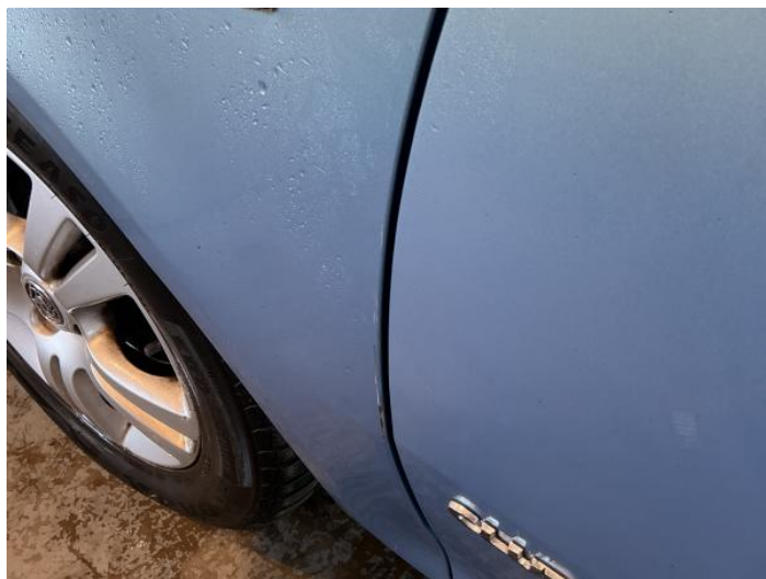
2: Wing nsf Scratched Over 25mm Thru Paint
