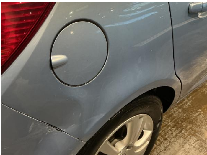
9: Qtr Panel osr Dented With Paint Damage
