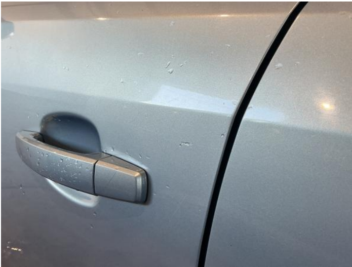
5: Door nsf Chipped Edge Chip
