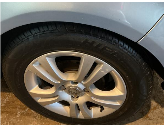
7: Wheel nsr Scratched Over 50mm
