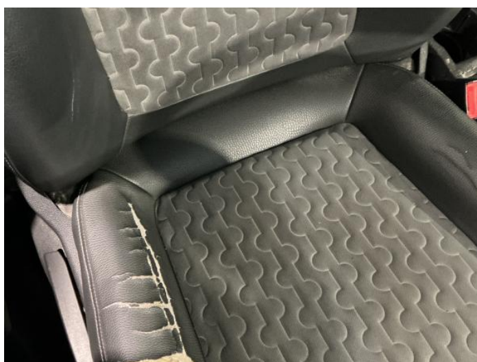
14: Seat Base Cover osf Scuffed Over 25mm
