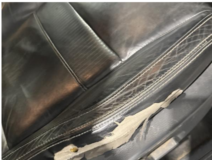
1: Seat Base Cover osf Torn Over 3mm
