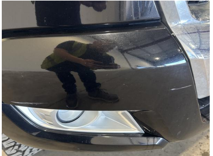
4: Bumper Front Scratched Over 100mm Thru Paint
