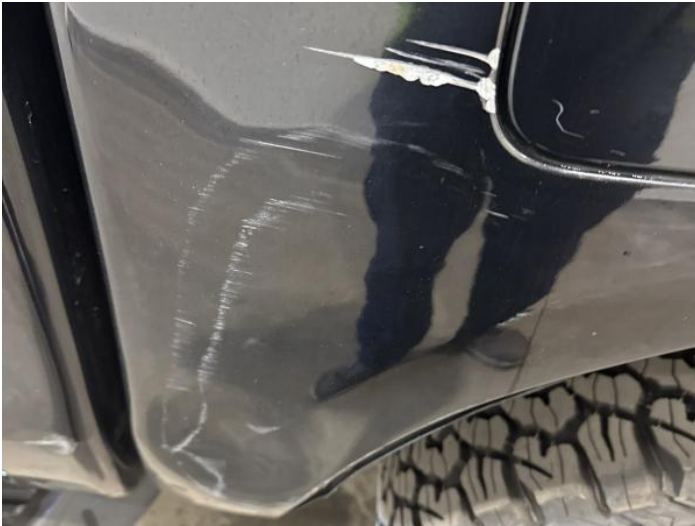
9: Qtr Panel nsr Dented With Paint Damage
