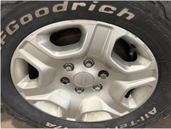
15: Wheel osr Scratched Over 50mm
