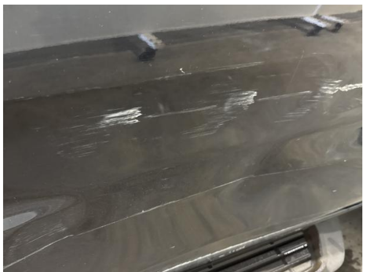
8: Door nsr Dented With Paint Damage
