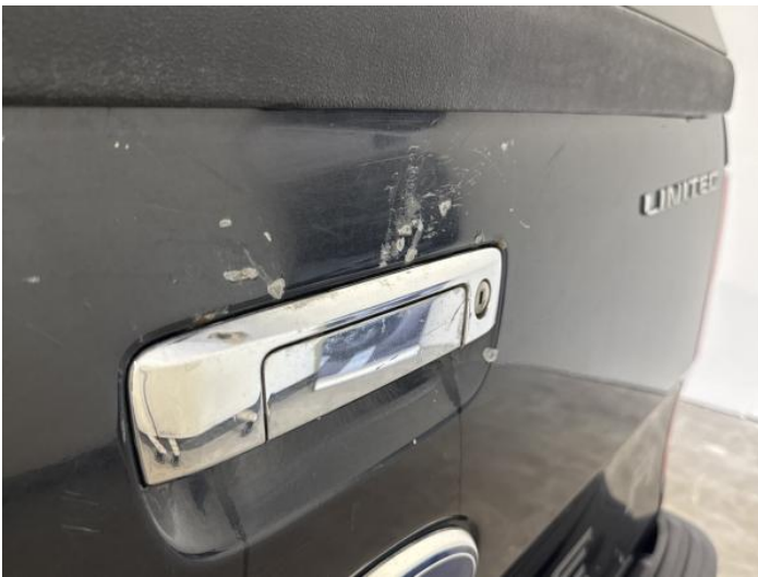
11: Boot Lid Dented With Paint Damage
