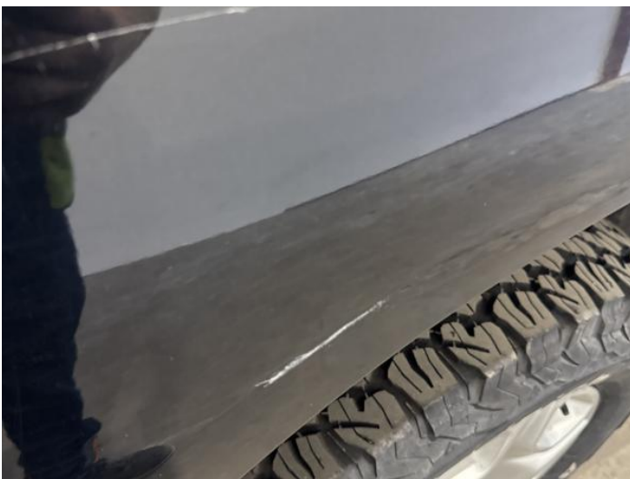
13: Qtr Panel osr Dented With Paint Damage
