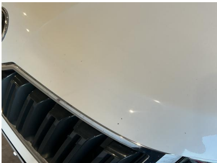
1: Bonnet Chipped Multiple Chips
