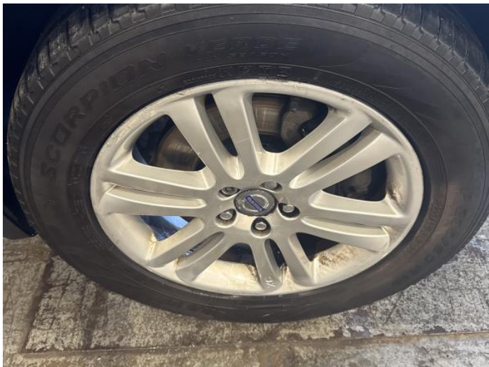
21: Wheel osf Scratched Over 50mm
