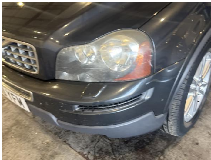
2: Bumper Front Scratched 25 to 100mm Thru Paint
