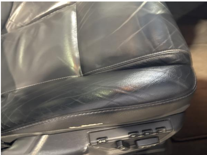
22: Seat Base Cover osf Torn Over 3mm
