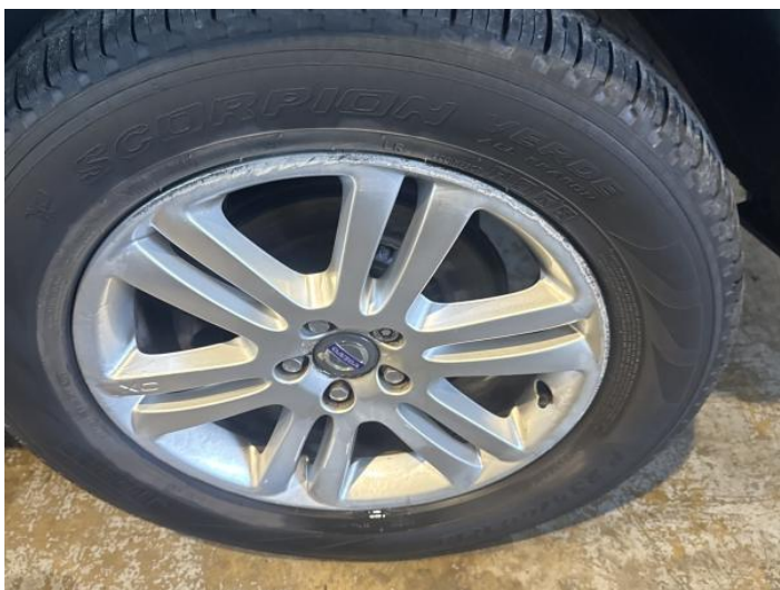
11: Wheel nsr Scratched Over 50mm
