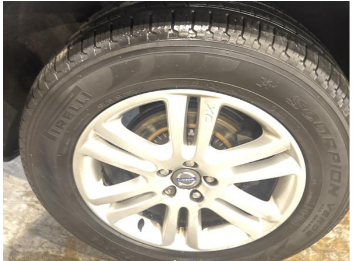
16: Wheel osr Scratched Up To 50mm
