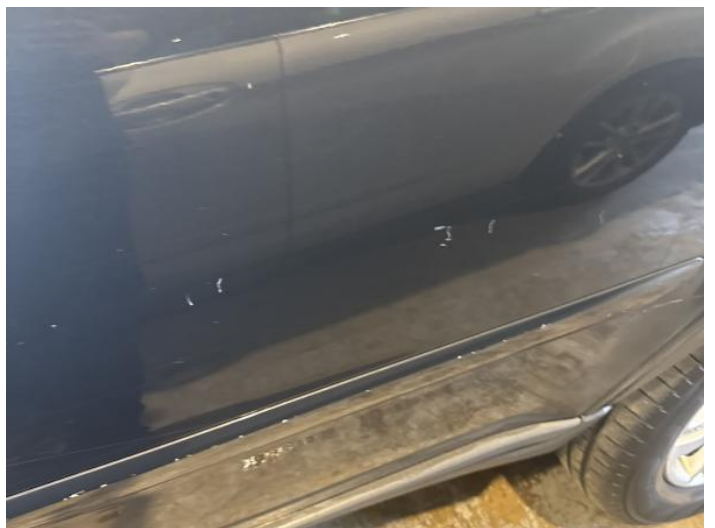
8: Door nsr Dented With Paint Damage
