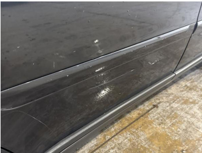
17: Door osr Dented With Paint Damage
