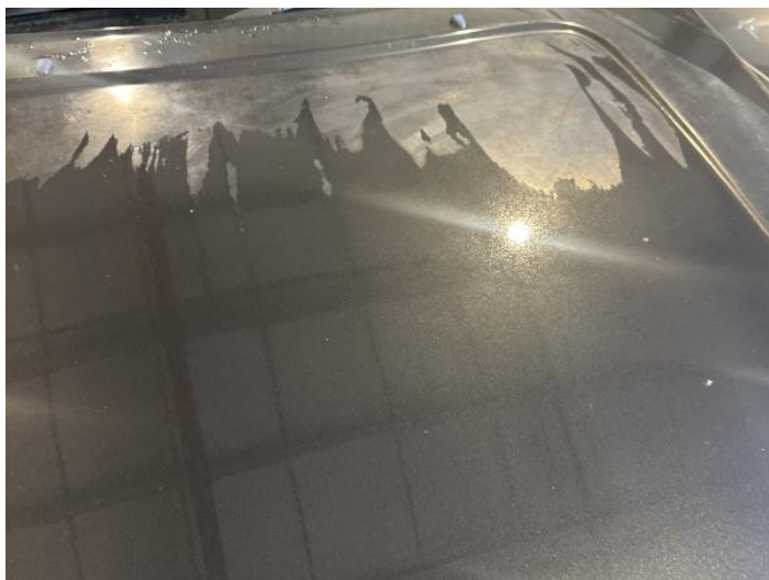
1: Bonnet Poor Previous Repair Poor Paint
