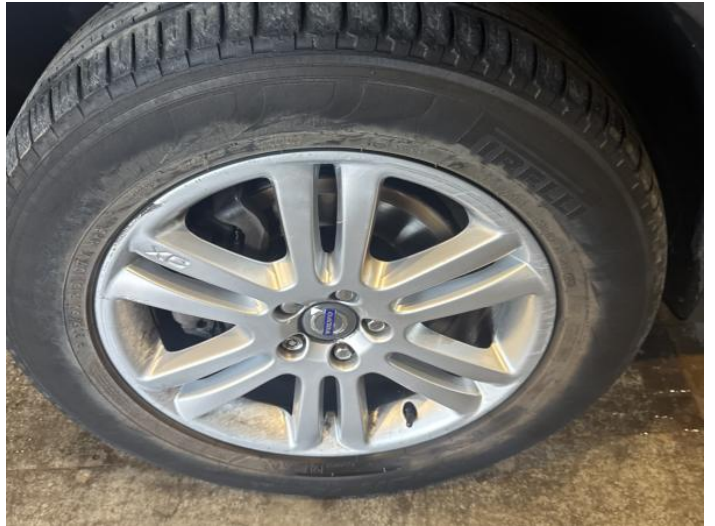
4: Wheel nsf Scratched Up To 50mm
