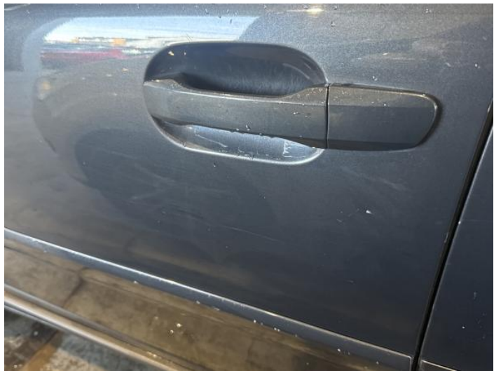
6: Door nsf Dented Over 2 UpTo 10mm
