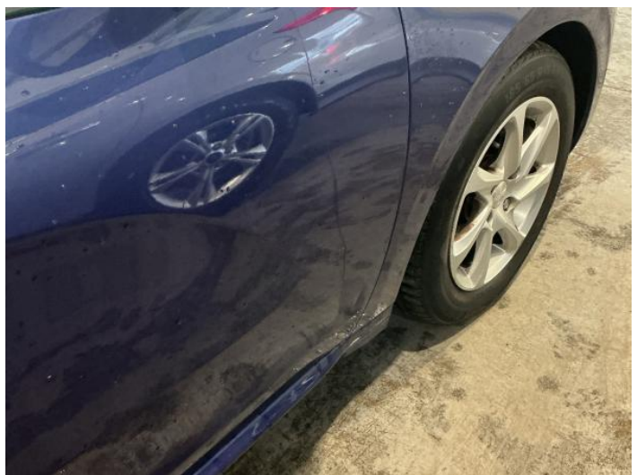
6: Door osf Dented Between 10mm + 30mm
