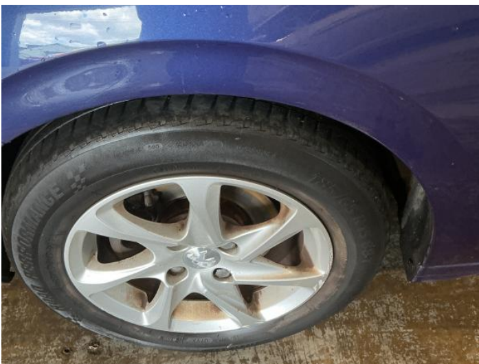
19: Wheel nsf Scratched Up To 50mm
