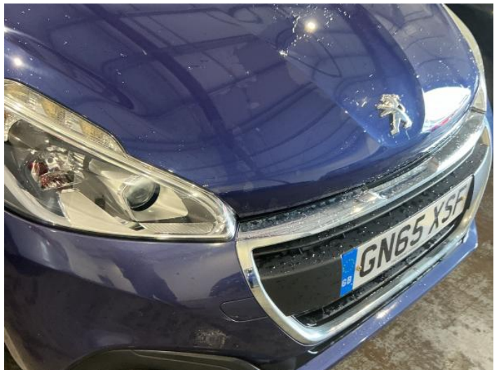
2: Bumper Front Poor Previous Repair Poor Paint
