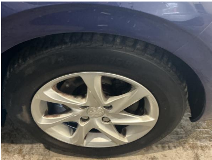
3: Wheel osf Scratched Up To 50mm
