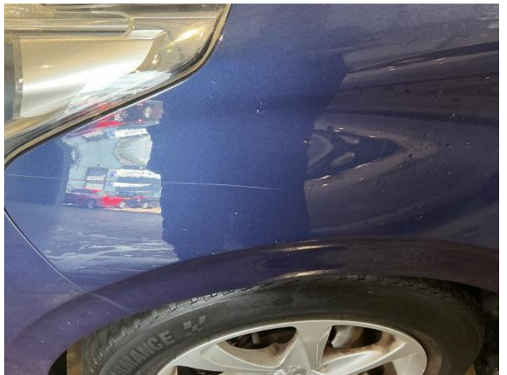
18: Wing nsf Scratched Over 25mm Thru Paint
