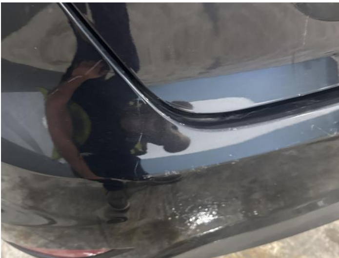
11: Bumper Rear Scratched Over 100mm Thru Paint
