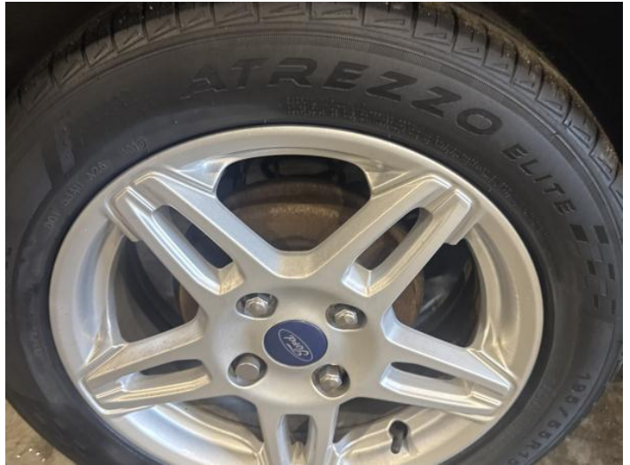
10: Wheel osr Scratched Up To 50mm
