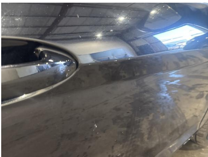
7: Door osf Dented With Paint Damage
