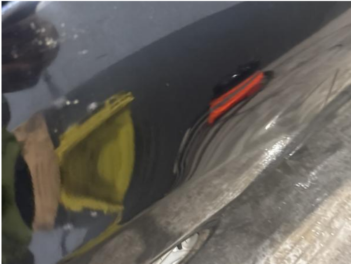
16: Wing nsf Scratched Over 25mm Not Thru Paint
