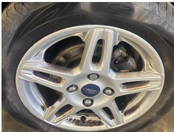
6: Wheel osf Scratched Over 50mm
