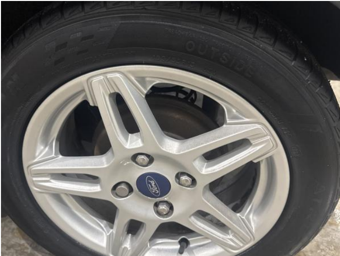
15: Wheel nsr Scratched Up To 50mm
