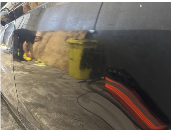
13: Door nsr Dented With Paint Damage
