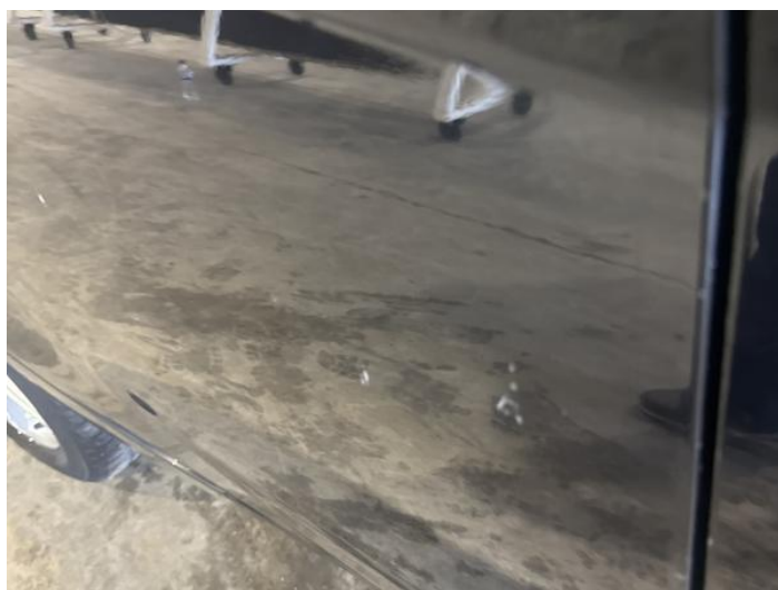
8: Door osf Dented With Paint Damage
