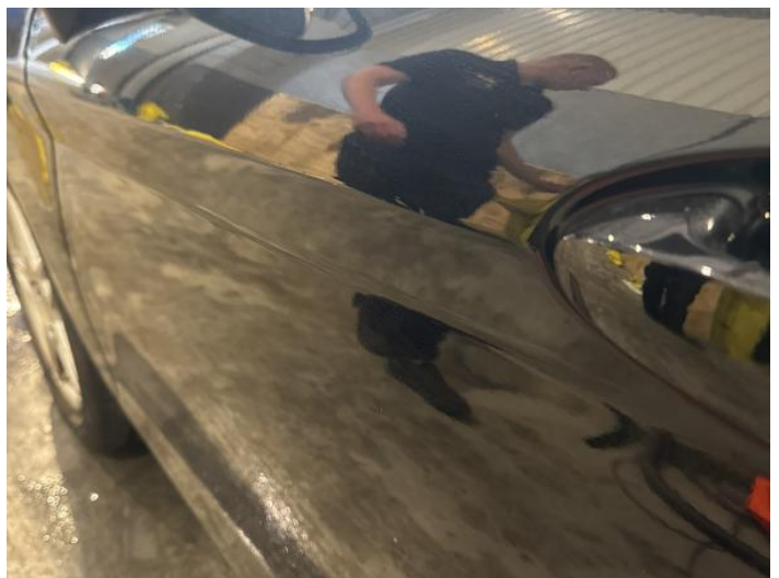
14: Door nsf Dented With Paint Damage
