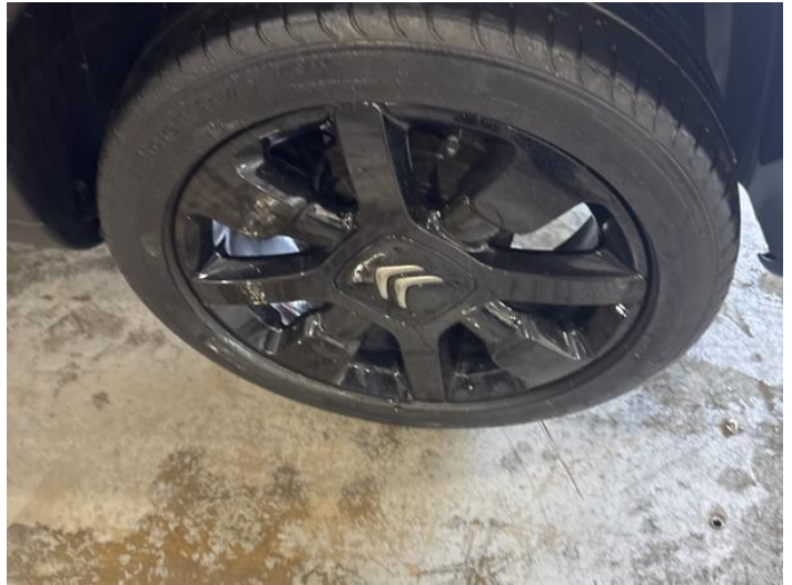
16: Wheel nsr Scratched Up To 50mm
