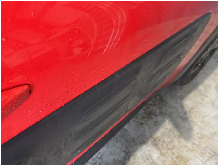
5: Door osf Dented Over 2 UpTo 10mm
