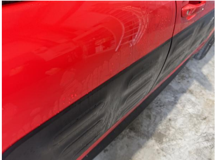
4: Door osr Dented Over 2 UpTo 10mm
