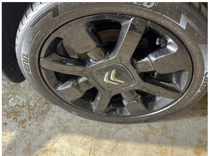
8: Wheel osf Scratched Up To 50mm
