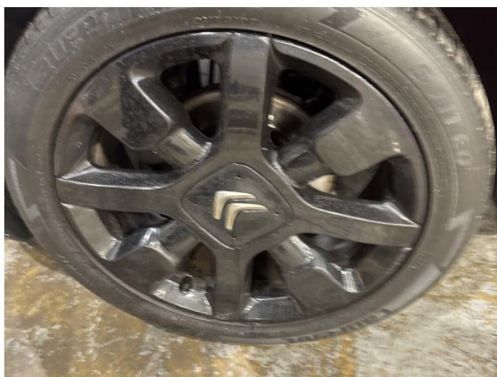
12: Wheel nsf Scratched Over 50mm
