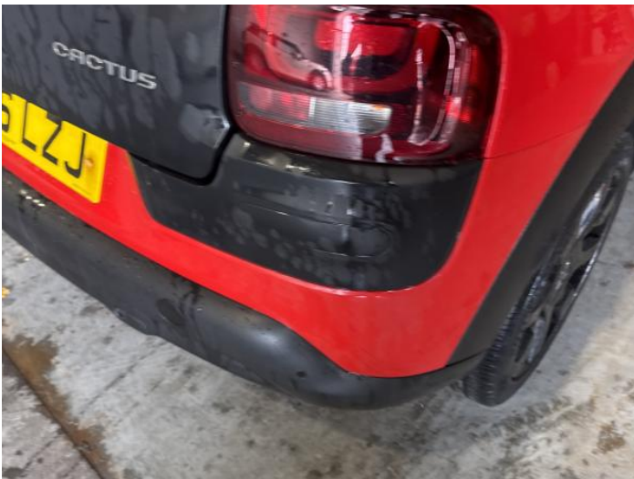
1: Bumper Rear Chipped Multiple Chips
