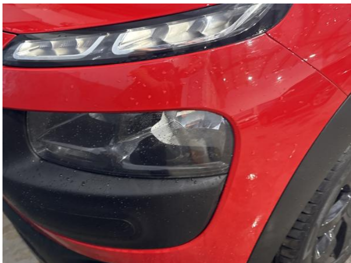
9: Bumper Front Scratched 25 to 100mm Thru Paint
