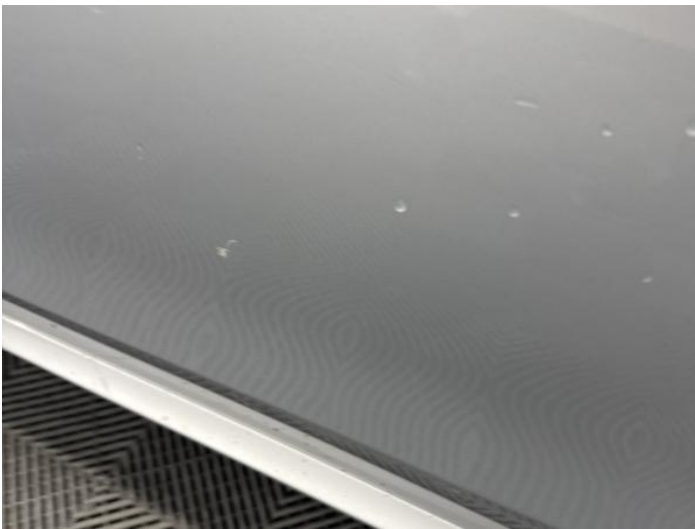
5: Door nsf Chipped Over 5mm
