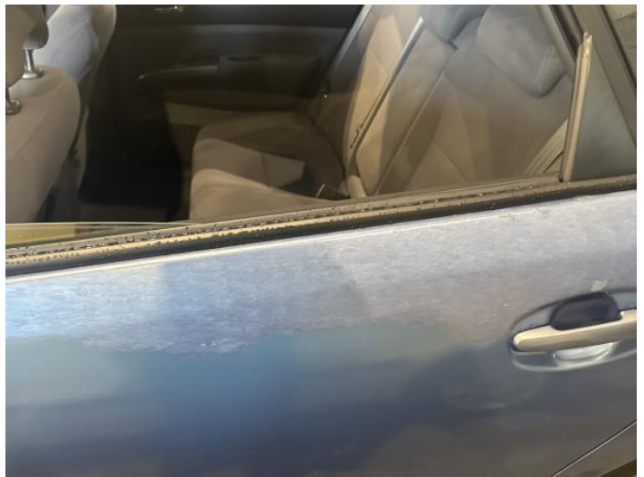
6: Door nsr Poor Previous Repair Poor Paint
