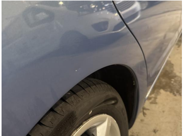
10: Qtr Panel osr Dented With Paint Damage
