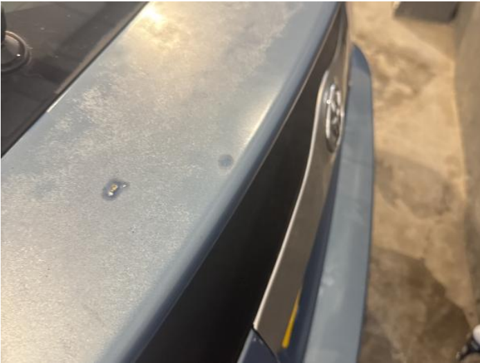
9: Boot Lid Poor Previous Repair Poor Paint
