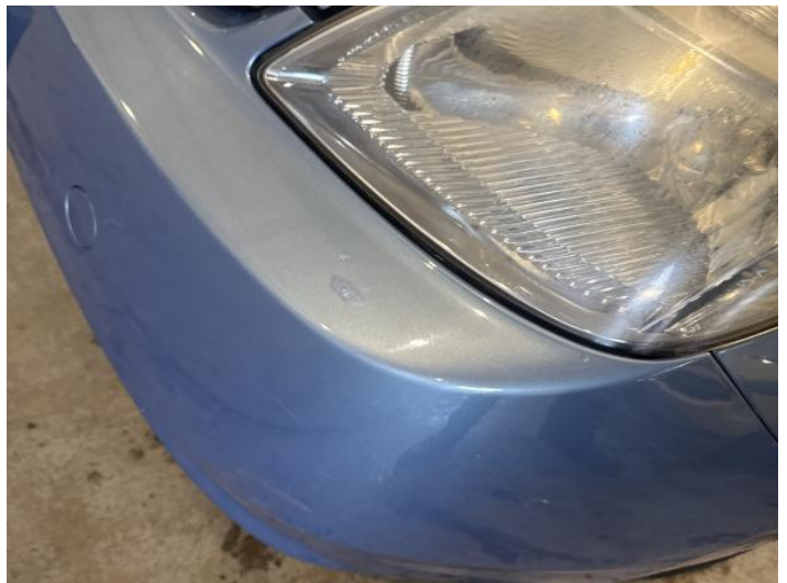
2: Bumper Front Poor Previous Repair Poor Paint
