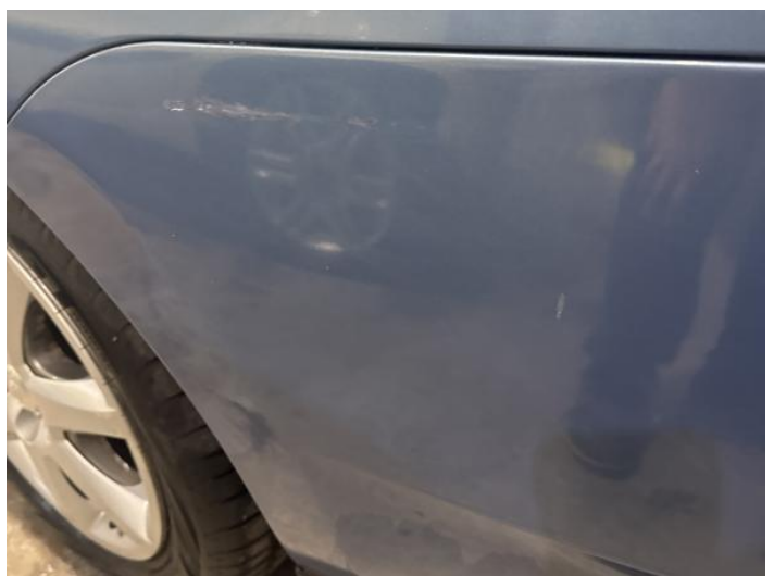
8: Bumper Rear Poor Previous Repair Poor Paint
