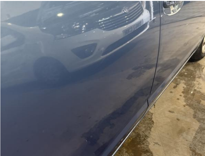
11: Door osr Poor Previous Repair Poor Paint
