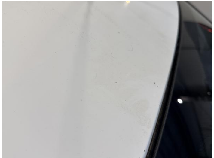
10: Roof Chipped Multiple Chips
