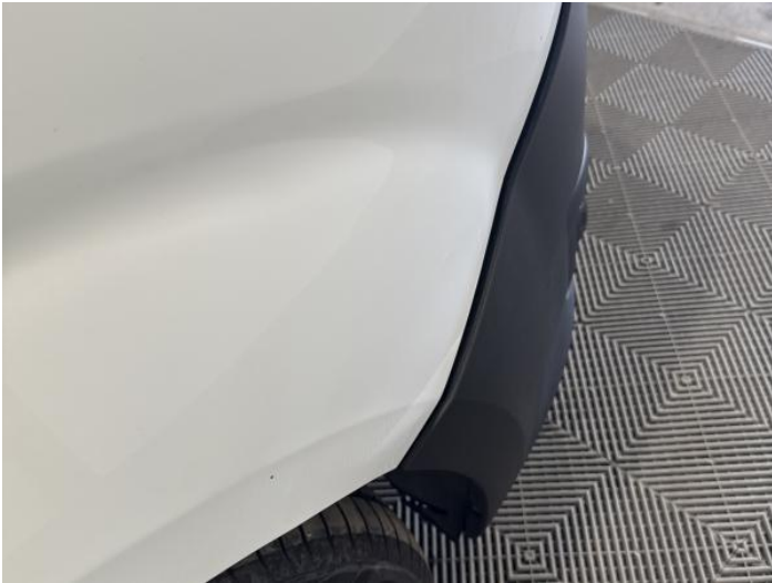
9: Wing osf Dented Over 30mm
