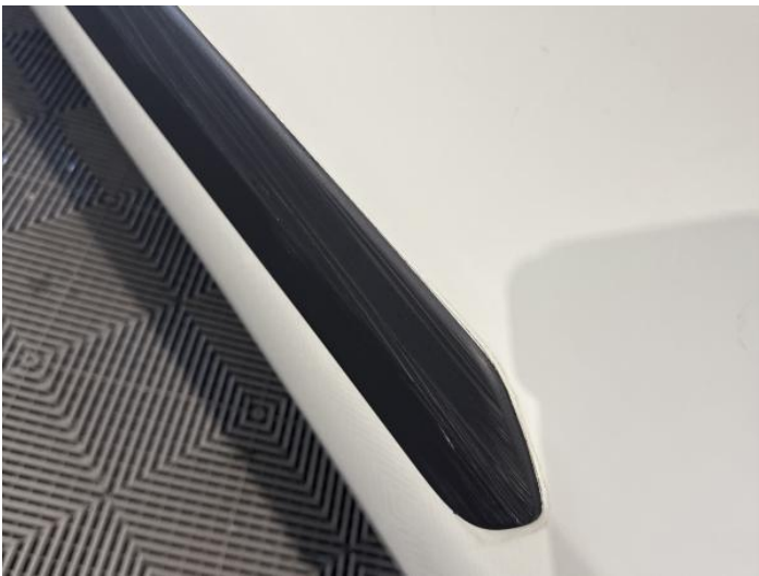
5: Door Moulding nsr Scuffed (Unpainted) Over 100mm
