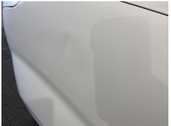
2: Wing nsf Dented Over 30mm
