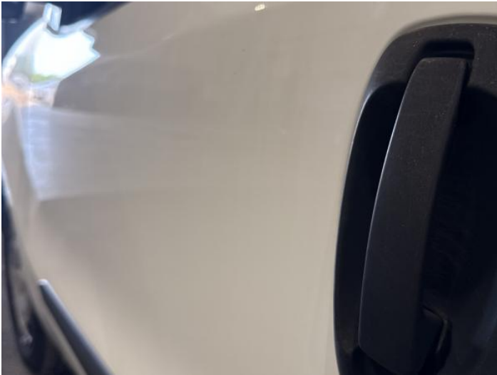
3: Door nsf Dented Between 10mm + 30mm
