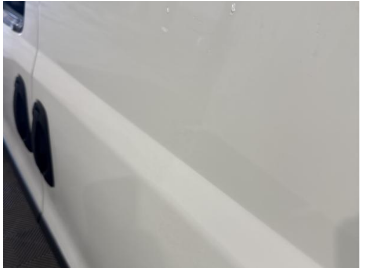
4: Door nsr Dented Over 30mm
