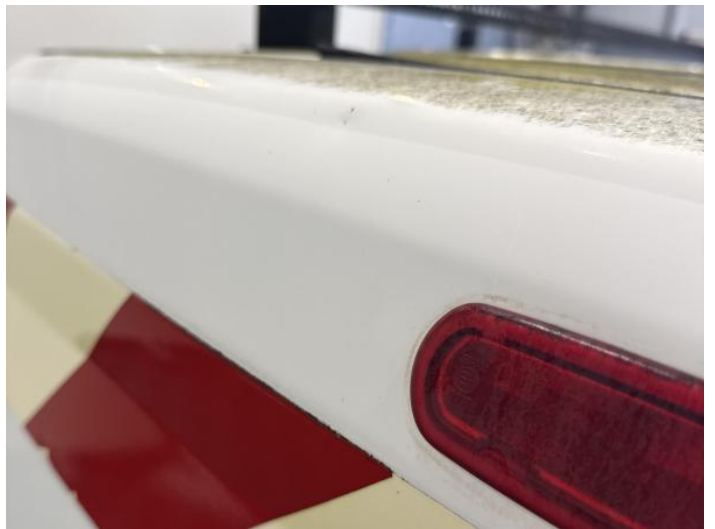
6: Tailgate Dented With Paint Damage
