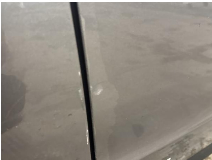
13: Door osr Scratched UpTo 25mm Thru Paint
