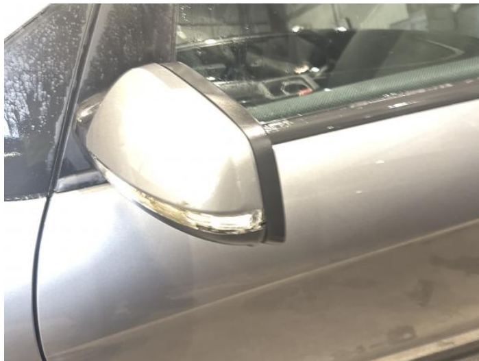
4: Door Mirror Assy nsf Broken Replace
