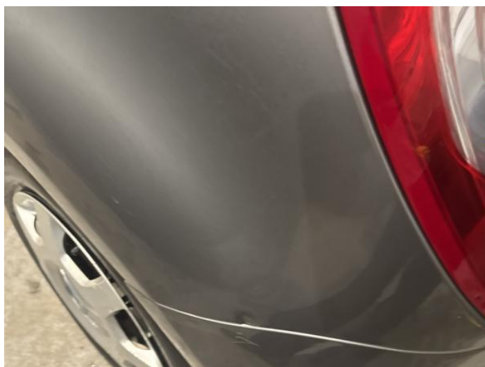
8: Qtr Panel nsr Dented Between 10mm + 30mm
