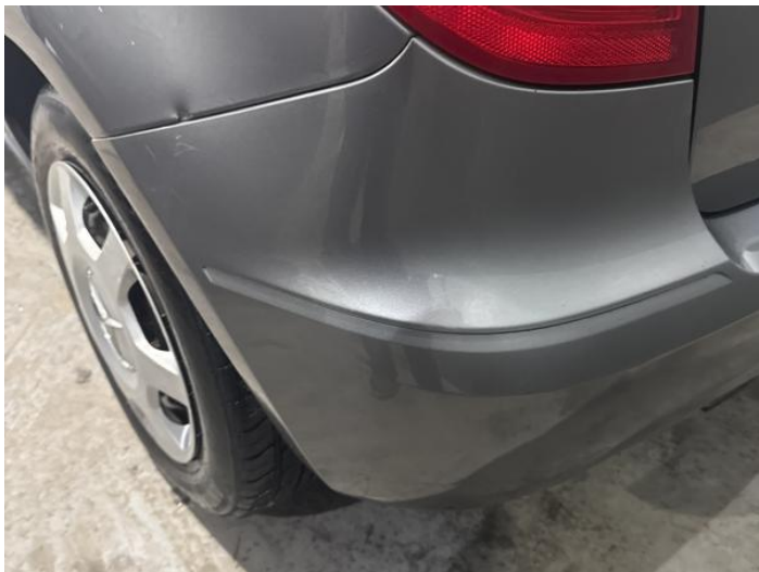
9: Bumper Rear Scratched Over 100mm Thru Paint
