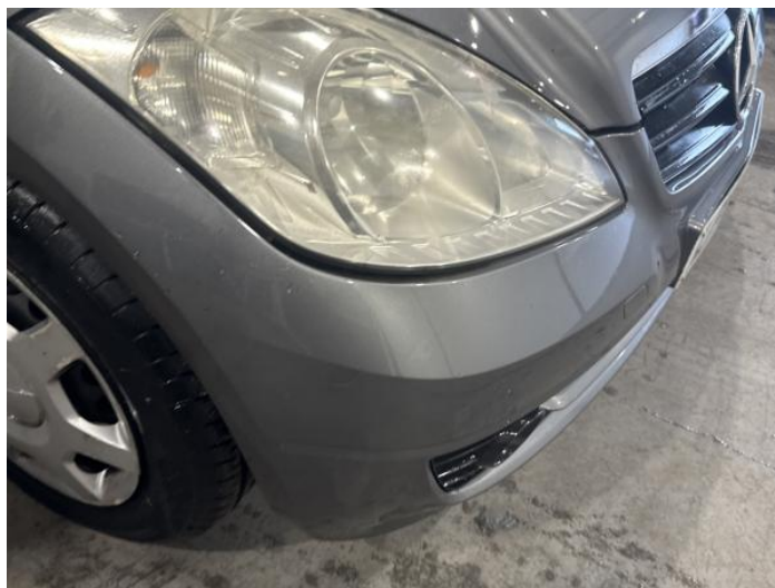
2: Bumper Front Scratched Over 100mm Thru Paint
