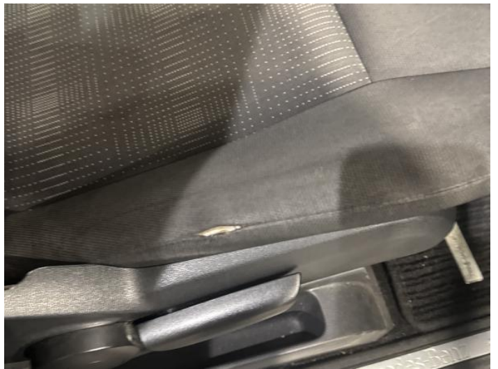
18: Seat Base Cover osf Torn Over 3mm
