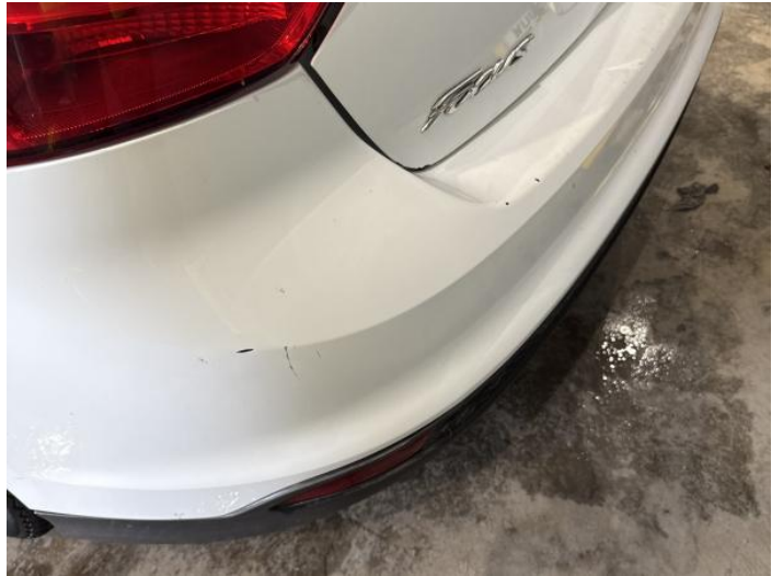
10: Bumper Rear Scratched Over 100mm Thru Paint
