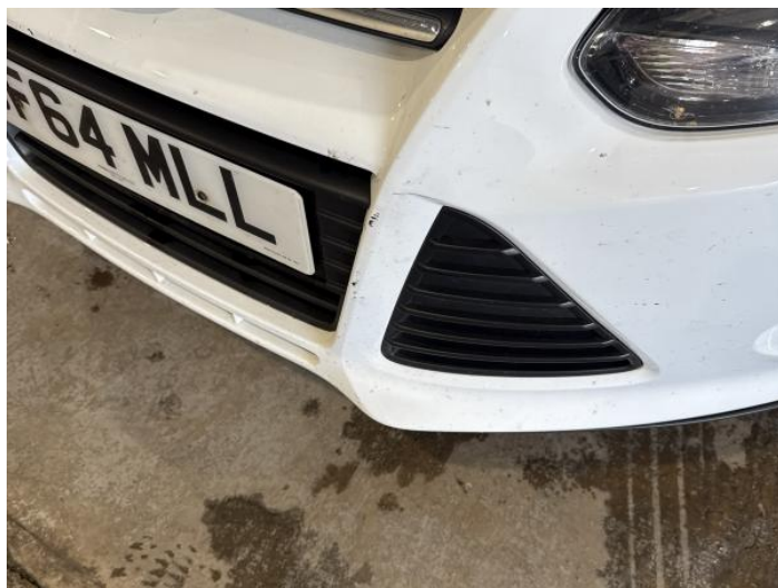
2: Bumper Front Scratched Over 100mm Thru Paint
