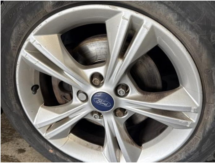
3: Wheel nsf Scratched Over 50mm
