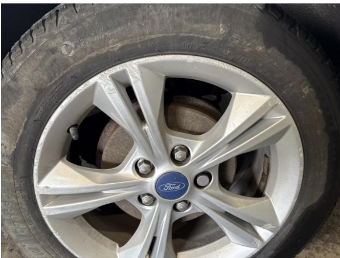
7: Wheel nsr Scratched Over 50mm
