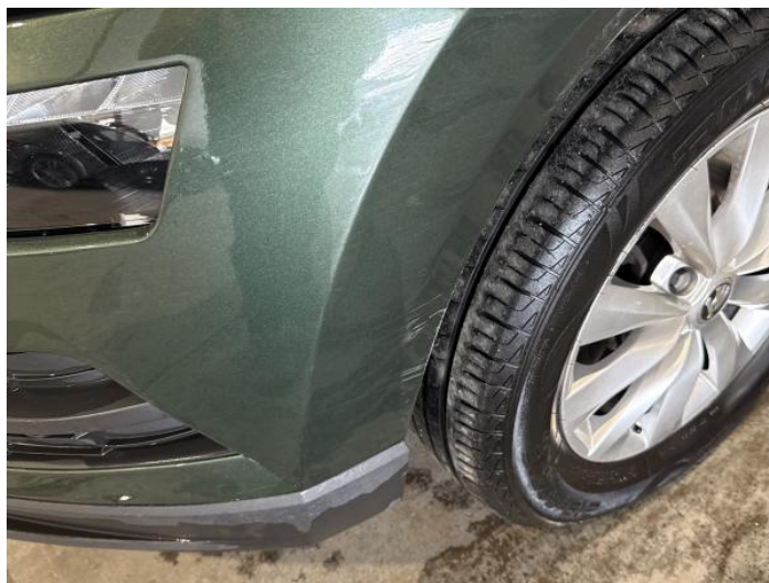
2: Bumper Front Scratched Over 100mm Thru Paint
