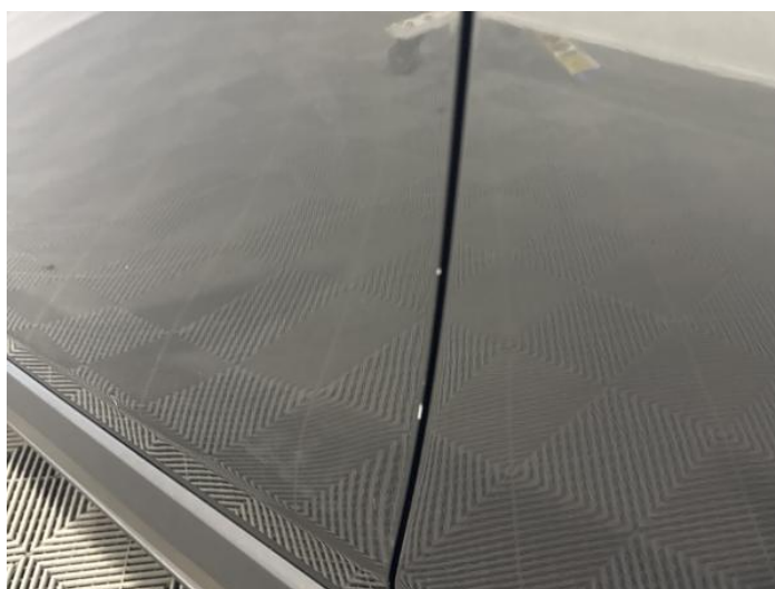
6: Door nsf Chipped Edge Chip
