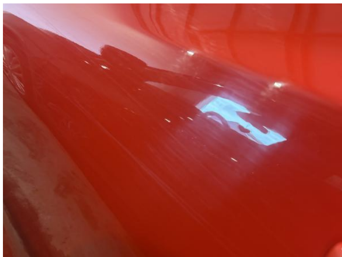
4: Door nsr Scratched Over 25mm Not Thru Paint
