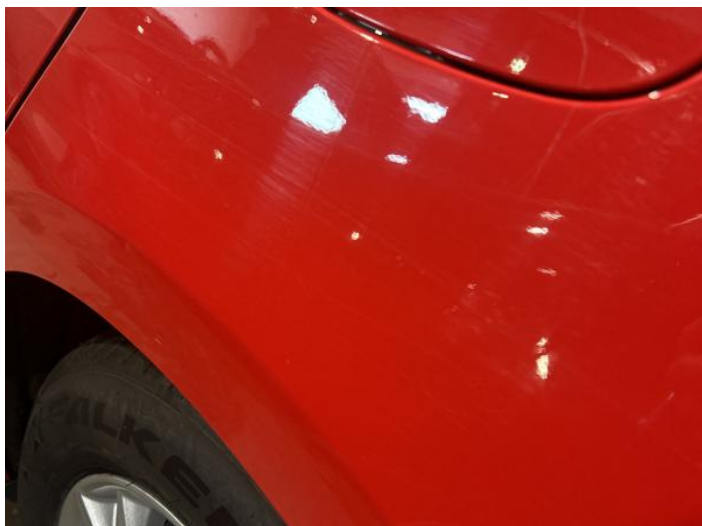
3: Qtr Panel nsr Scratched Over 25mm Not Thru Paint
