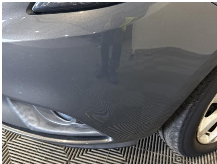
2: Bumper Front Scratched 25 to 100mm Thru Paint
