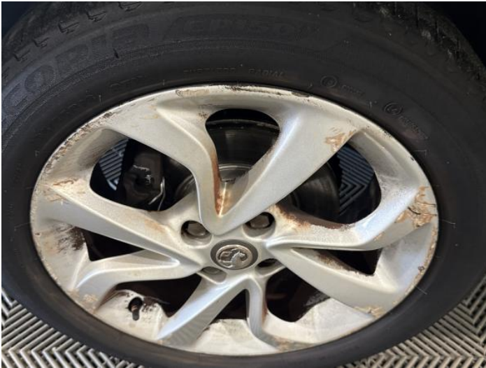
3: Wheel nsf Scratched Over 50mm
