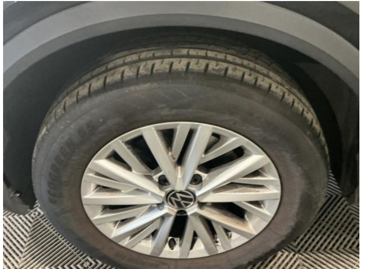
4: Wheel nsf Scratched Over 50mm
