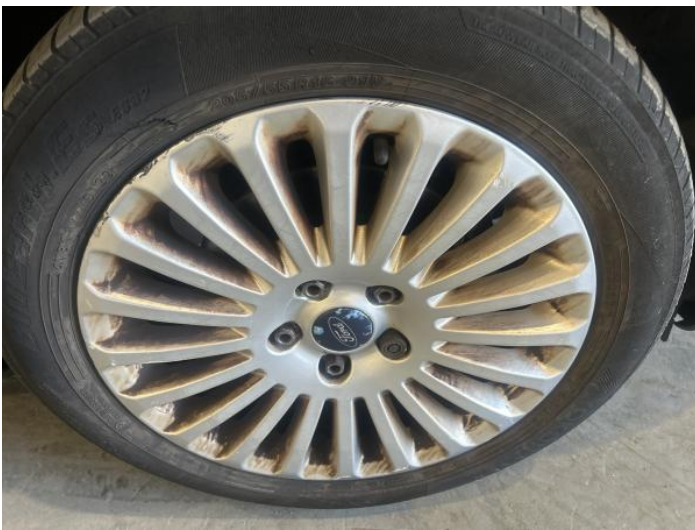
17: Wheel osf Scratched Over 50mm
