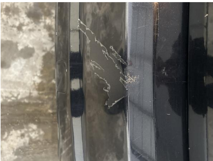
7: Bumper Rear Poor Previous Repair Paint Flake
