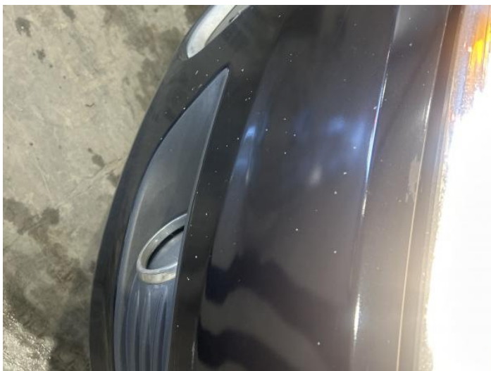
13: Bumper Front Poor Previous Repair Poor Paint
