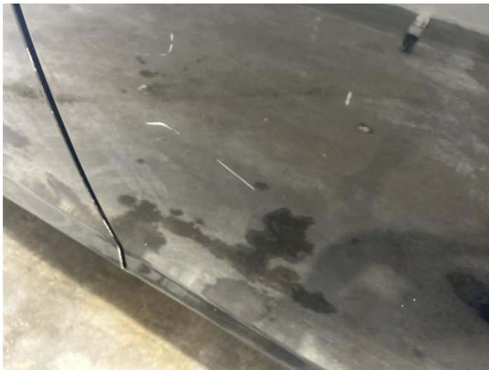
9: Door nsr Scratched Over 25mm Thru Paint
