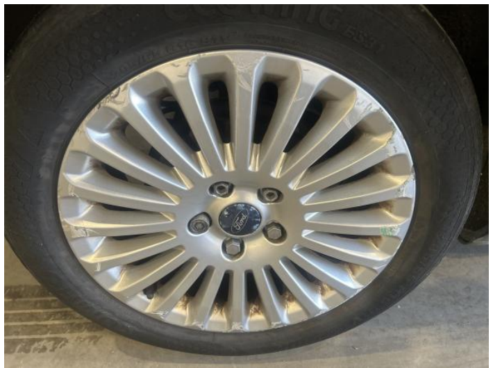
18: Wheel osr Scratched Over 50mm
