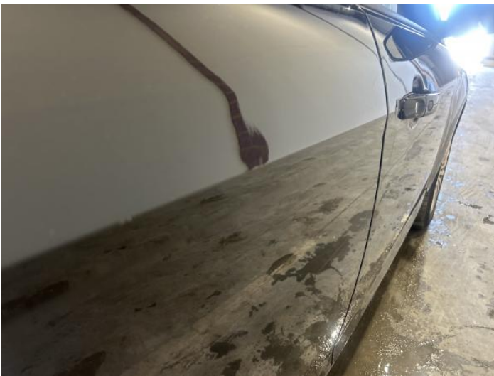
5: Door osr Dented 2 Or Less UpTo 10mm
