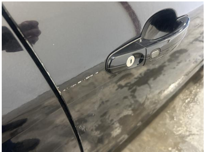
2: Door osf Scratched Over 25mm Thru Paint
