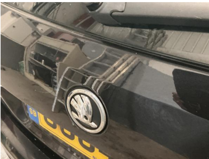
13: Boot Lid Dented Between 10mm + 30mm
