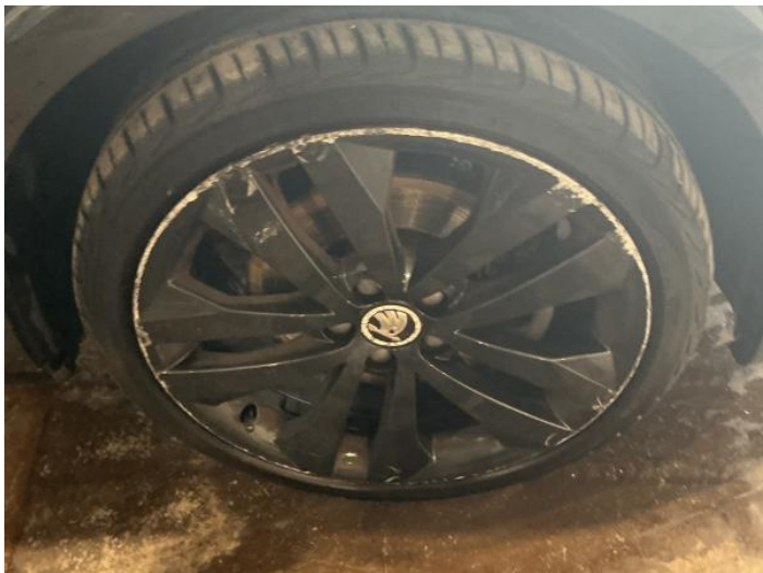
21: Wheel osf Scratched Over 50mm
