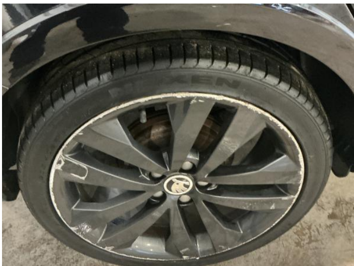
15: Wheel osr Scratched Over 50mm
