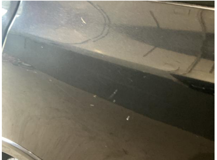
10: Qtr Panel nsr Dented Over 2 UpTo 10mm
