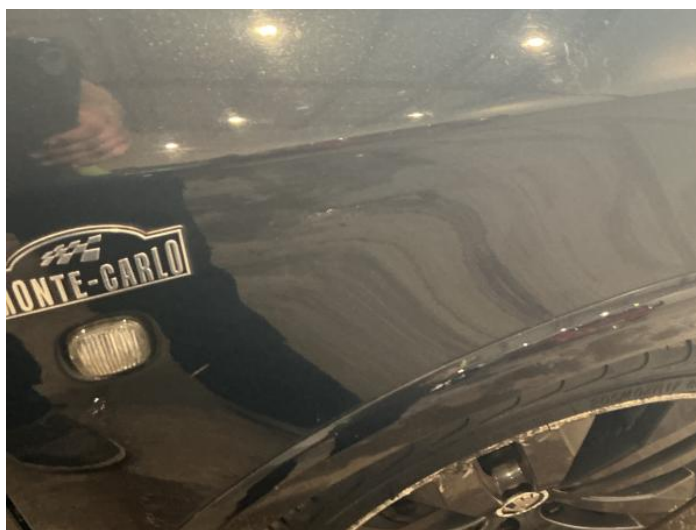
20: Wing osf Scratched UpTo 25mm Thru Paint
