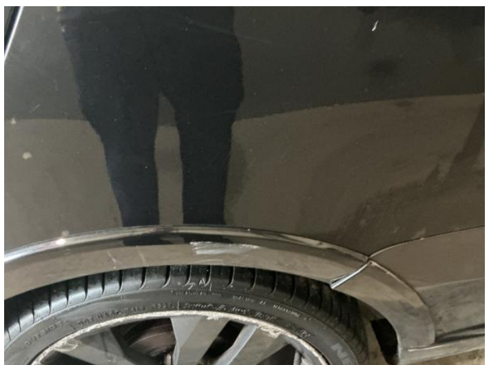
8: Qtr Panel Arch Extension ns Scratched (Painted) Over 25mm Thru Paint
