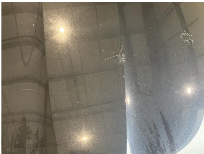
1: Bonnet Chipped Multiple Chips
