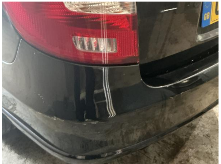
12: Bumper Rear Scratched Over 100mm Thru Paint
