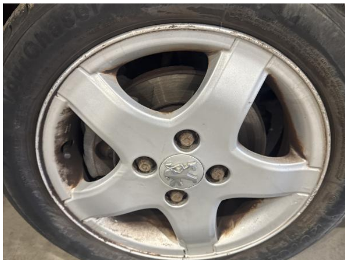
4: Wheel nsf Scratched Over 50mm
