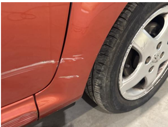
13: Wing osf Scratched Over 25mm Thru Paint
