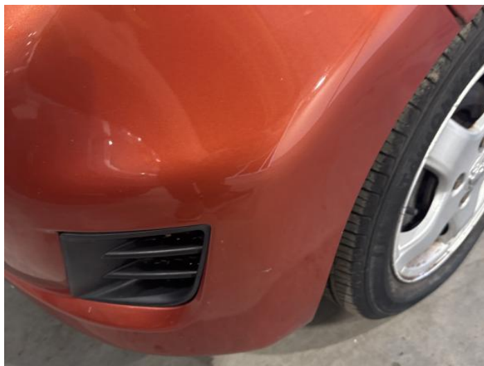
2: Bumper Front Scratched 25 to 100mm Thru Paint
