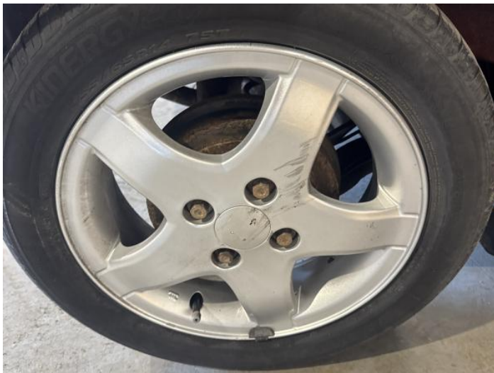
9: Wheel osr Scratched Over 50mm
