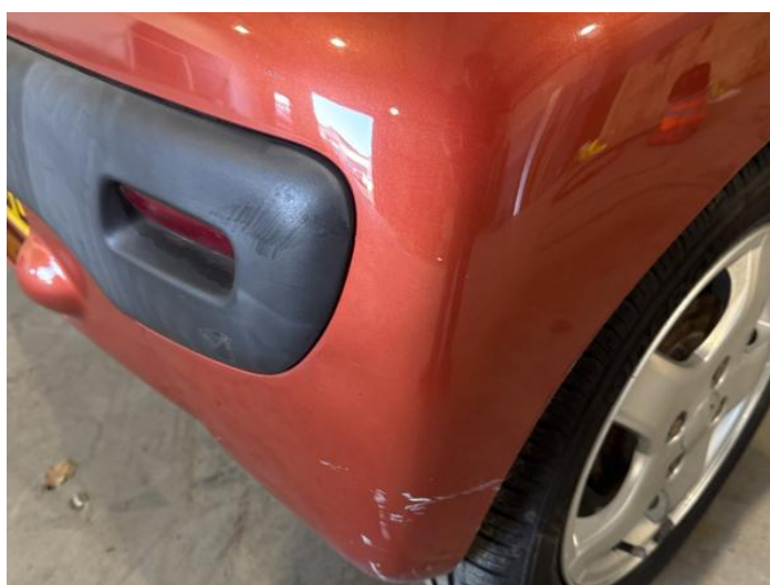
8: Bumper Rear Scratched Over 100mm Thru Paint
