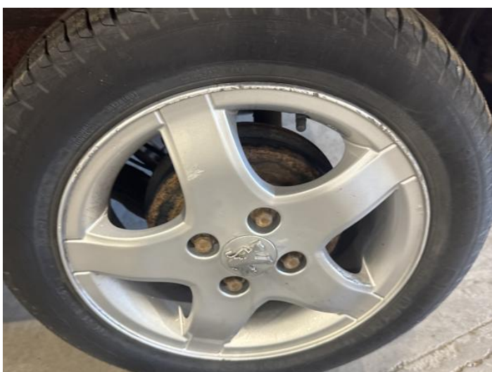
7: Wheel nsr Scratched Over 50mm
