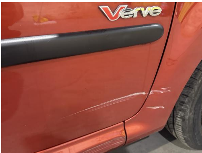
11: Door osf Scratched Over 25mm Thru Paint
