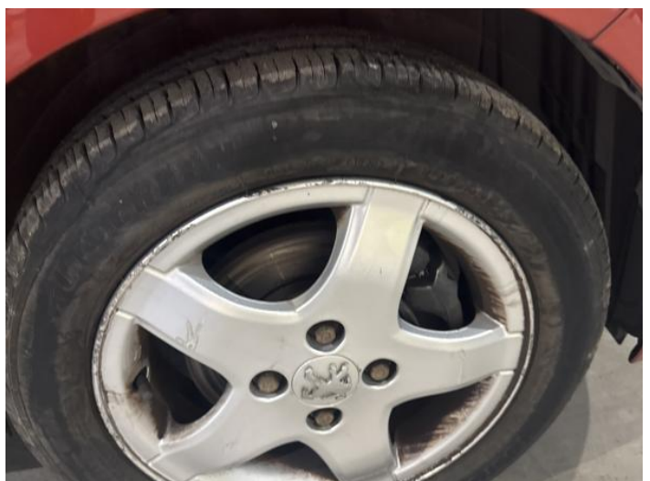
14: Wheel osf Scratched Over 50mm
