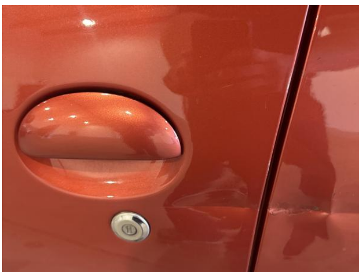
5: Door nsf Dented Over 30mm
