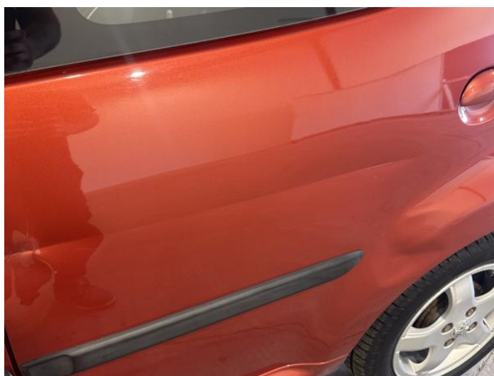
6: Door nsr Dented Over 30mm
