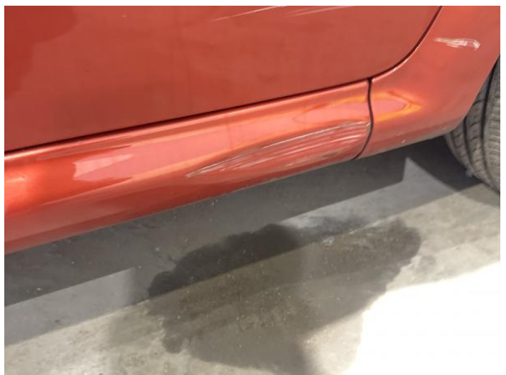
12: Sill os Dented With Paint Damage
