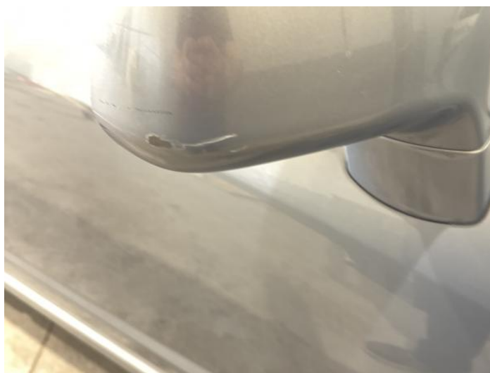
14: Door Mirror Assy osf Scratched (Painted) Over 25mm Thru Paint
