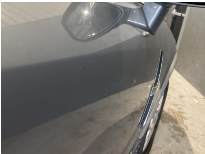
15: Door osf Dented Over 2 UpTo 10mm
