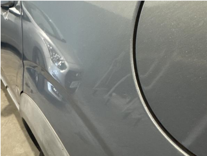
3: Qtr Panel nsr Dented Over 2 UpTo 10mm
