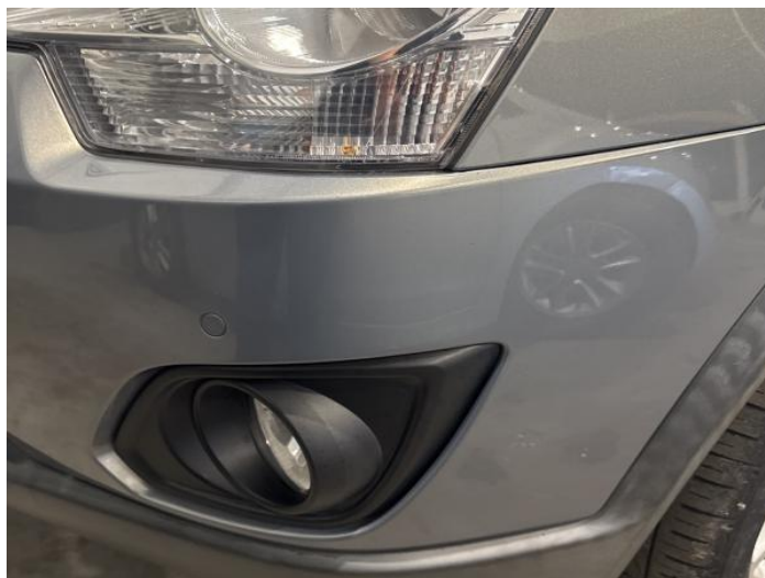
10: Bumper Front Scratched 25 to 100mm Thru Paint
