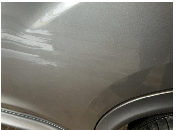
8: Door nsr Dented With Paint Damage
