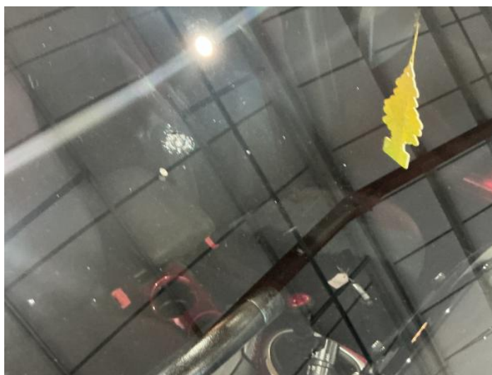
20: Screen Front Chipped UpTo 10mm
