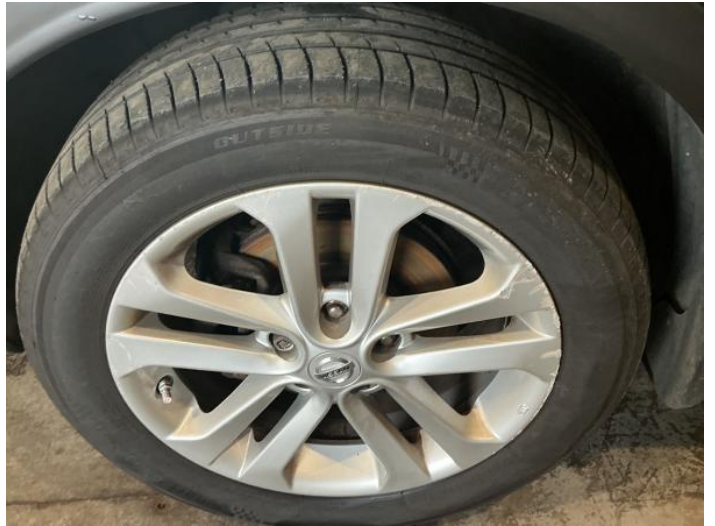
4: Wheel nsf Scratched Over 50mm
