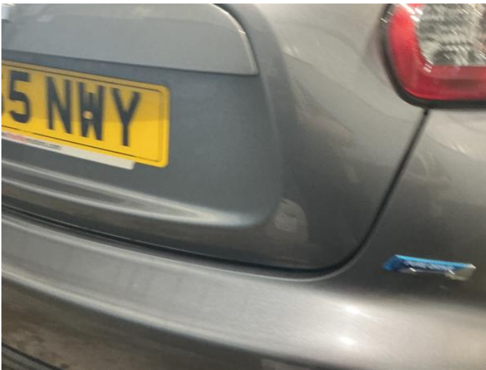
11: Bumper Rear Chipped Multiple Chips
