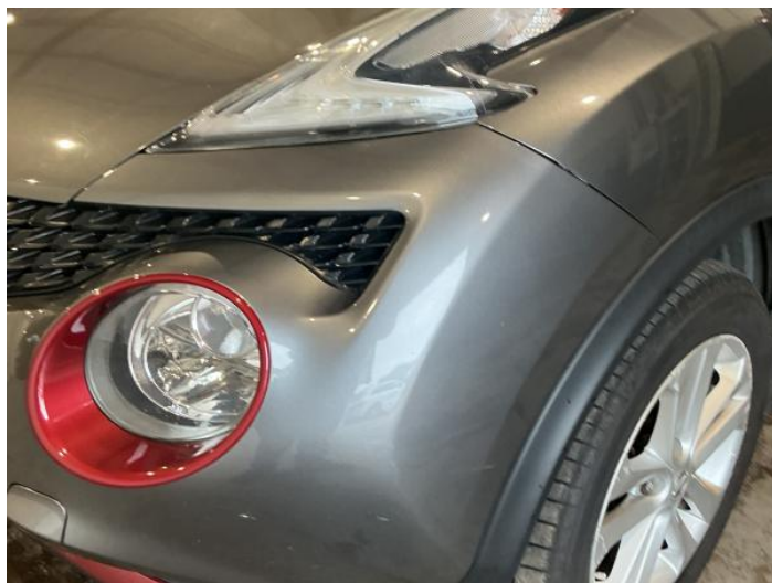
2: Bumper Front Scratched 25 to 100mm Thru Paint
