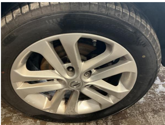
19: Wheel osf Scratched Up To 50mm
