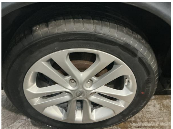
14: Wheel osr Scratched Up To 50mm
