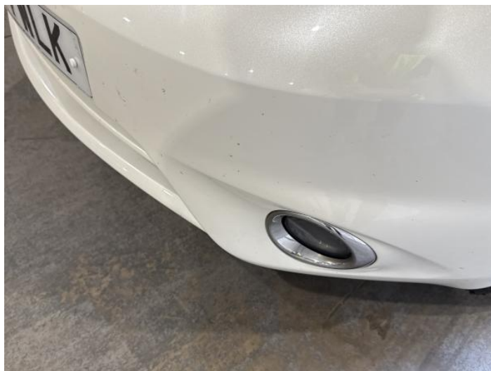
2: Bumper Front Chipped Multiple Chips
