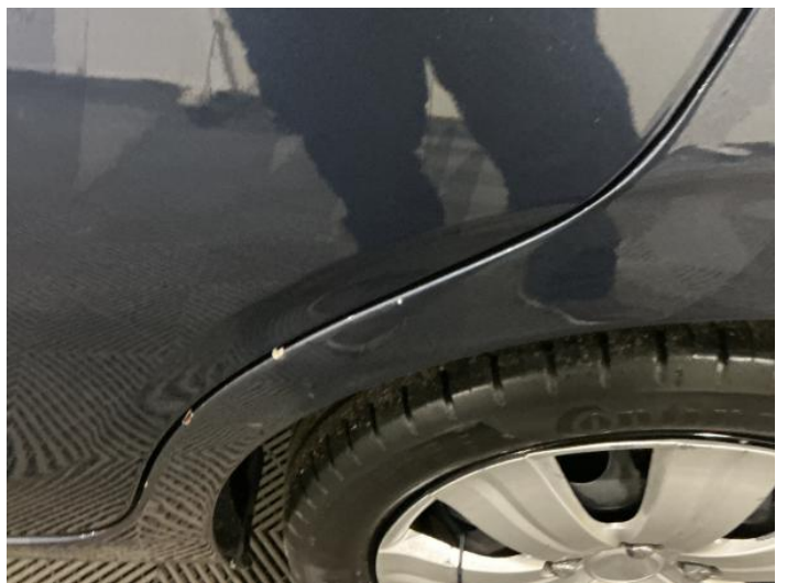
8: Qtr Panel nsr Rusted UpTo 5mm
