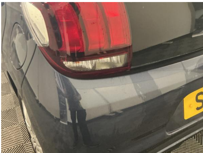
9: Bumper Rear Scratched 25 to 100mm Thru Paint
