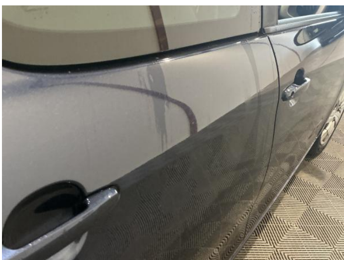
13: Door osr Dented Between 10mm + 30mm
