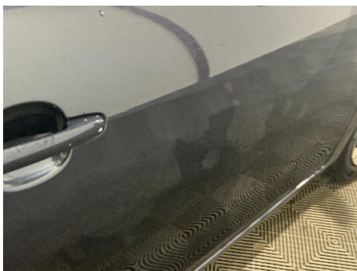
14: Door osf Dented Over 2 UpTo 10mm
