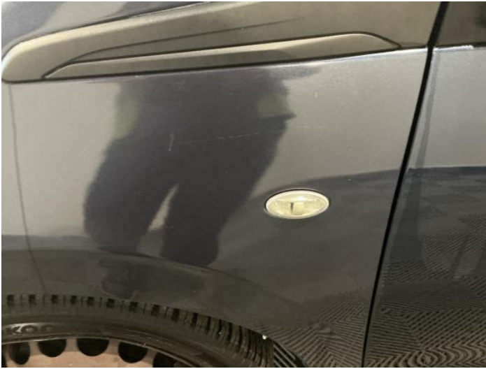
3: Wing nsf Poor Previous Repair Poor Paint
