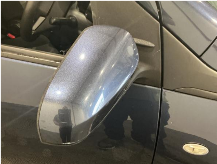
15: Door Mirror Assy osf Scratched (Painted) UpTo 25mm Thru Paint
