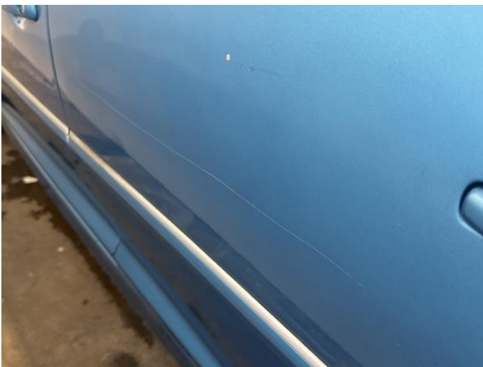
7: Door nsr Scratched Over 25mm Thru Paint
