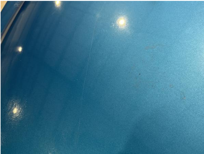
1: Bonnet Scratched Over 25mm Thru Paint
