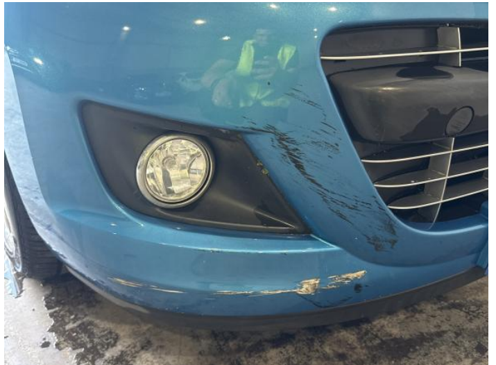
2: Bumper Front Scratched Over 100mm Thru Paint
