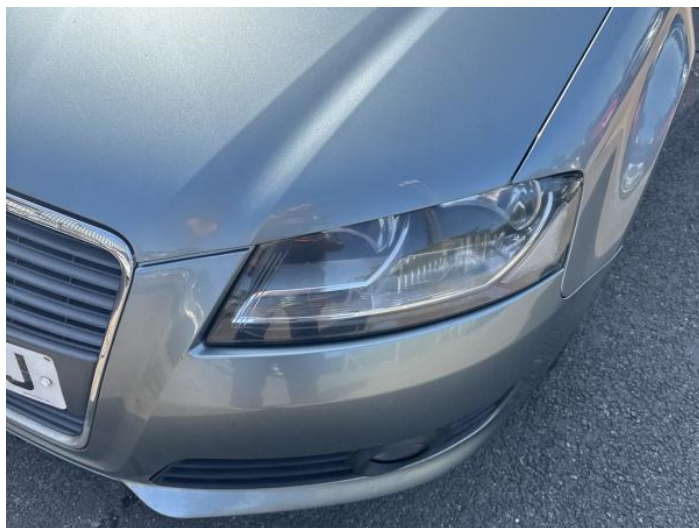
2: Bumper Front Poor Previous Repair Poor Paint
