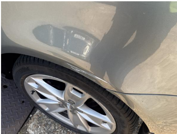
9: Qtr Panel nsr Dented With Paint Damage
