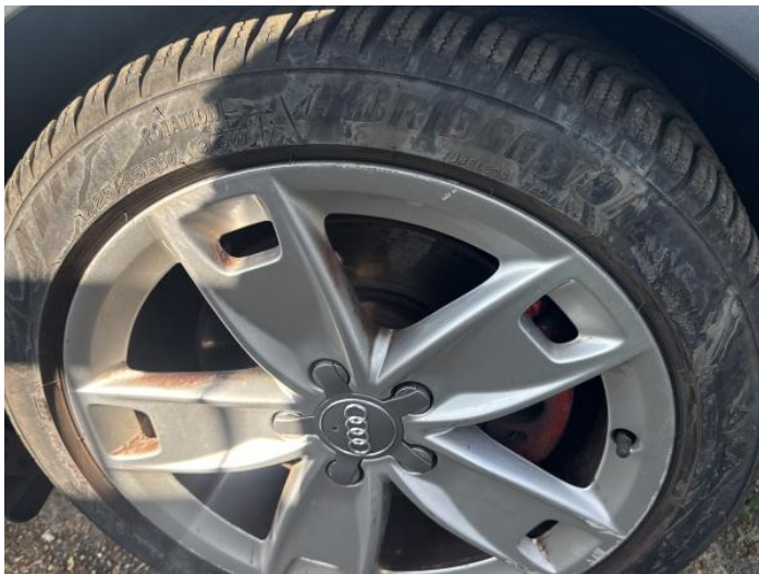
21: Wheel of Scratched Over 50mm
