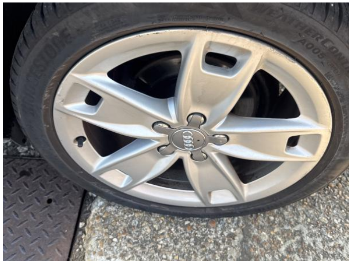
10: Wheel nsr Scratched Over 50mm
