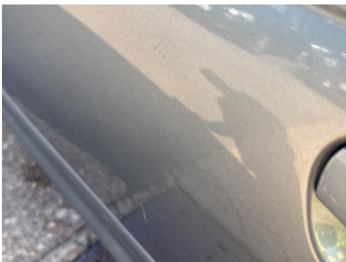
7: Door nsr Dented 2 Or Less UpTo 10mm
