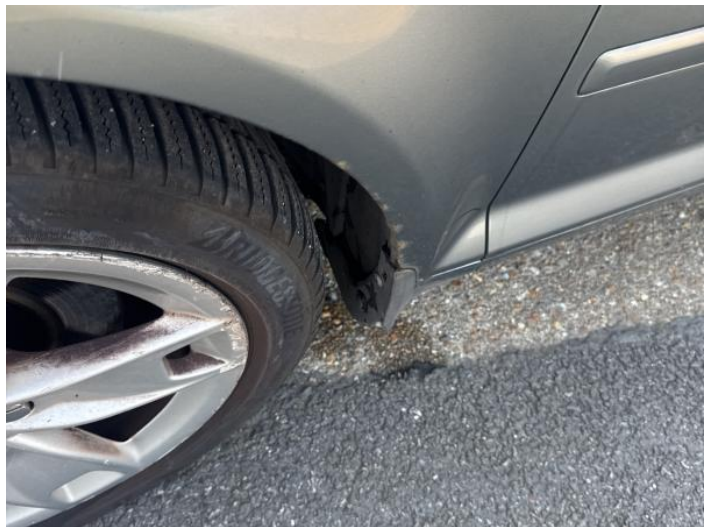
4: Wing nsf Rusted Over 5mm
