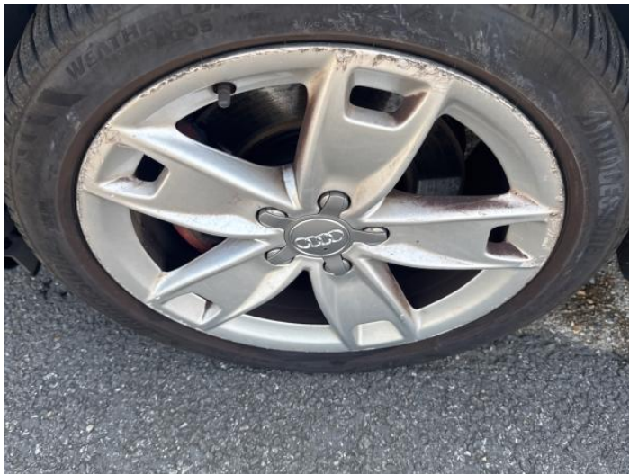
3: Wheel nsf Scratched Over 50mm
