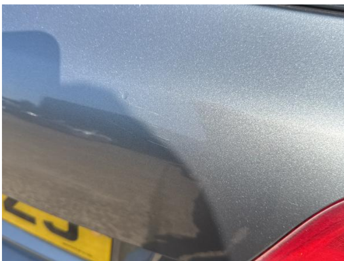
13: Boot Lid Scratched UpTo 25mm Thru Paint
