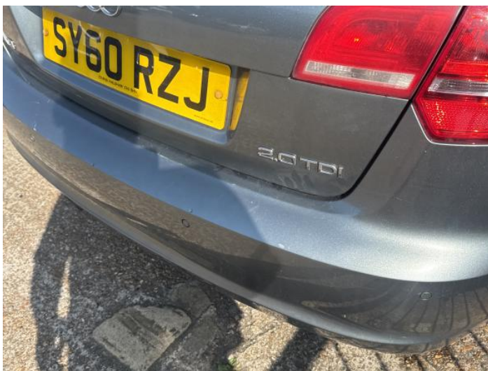
11: Bumper Rear Scratched 25 to 100mm Thru Paint
