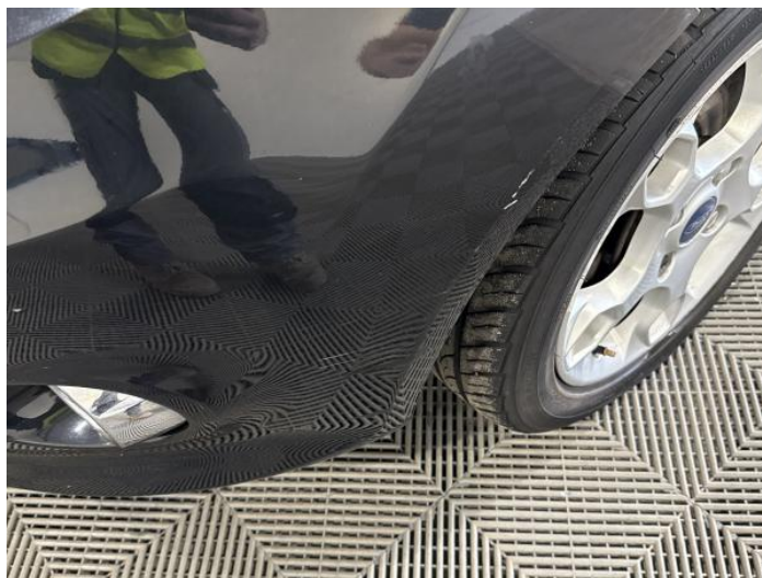
2: Bumper Front Scratched Over 100mm Thru Paint
