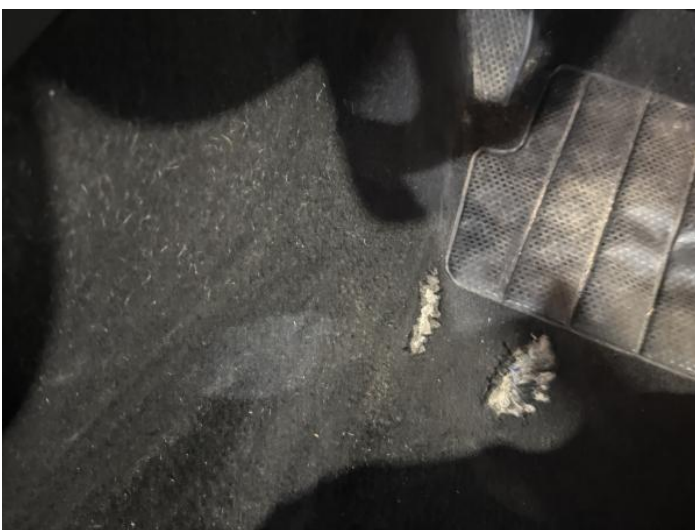
25: Carpets Front Torn Over 10mm
