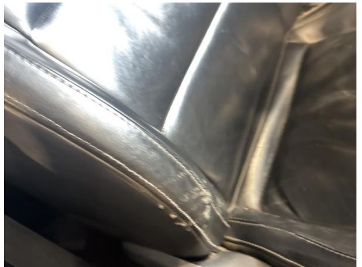
24: Seat Back Cover osf Torn UpTo 3mm
