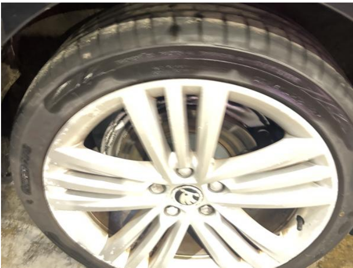
17: Wheel osr Scratched Over 50mm
