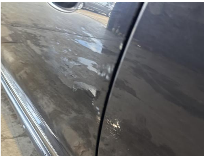
7: Door nsf Scratched UpTo 25mm Thru Paint
