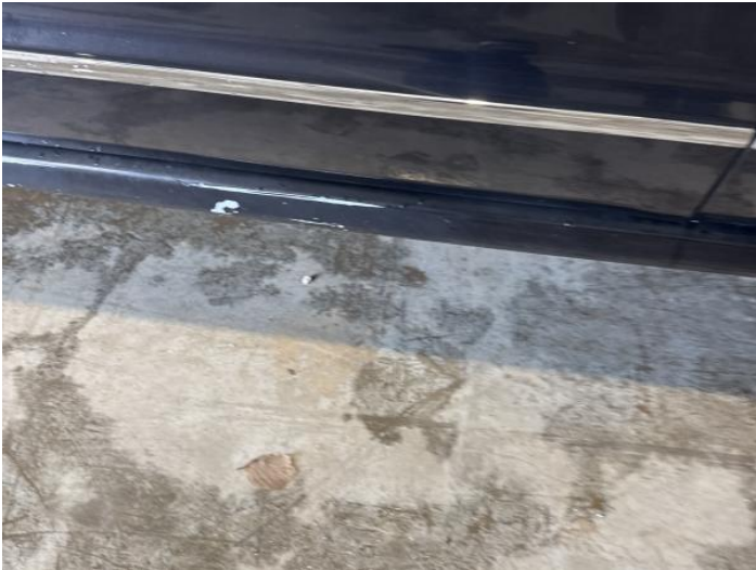
9: Sill ns Scratched Over 25mm Thru Paint
