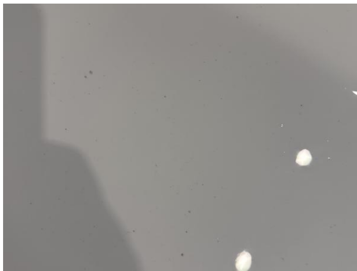
2: Bonnet Chipped Multiple Chips
