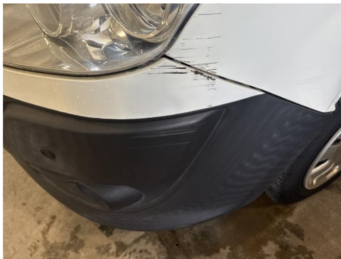
2: Bumper Front Scratched Over 100mm Thru Paint
