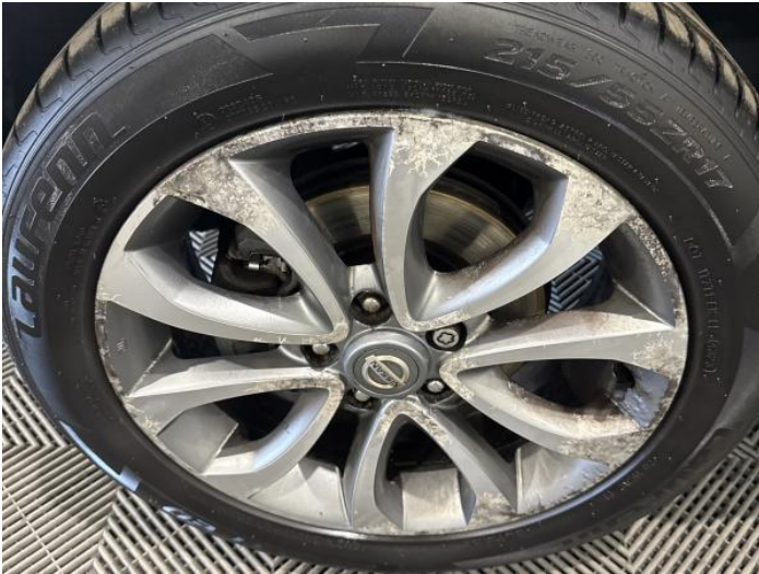
3: Wheel nsf Scratched Over 50mm
