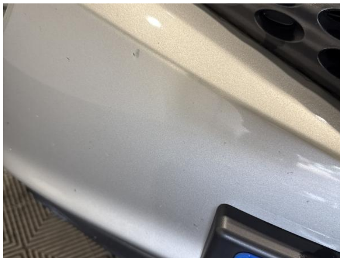
2: Bumper Front Chipped Multiple Chips
