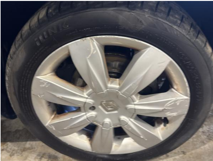
23: Wheel osf Scratched Over 50mm
