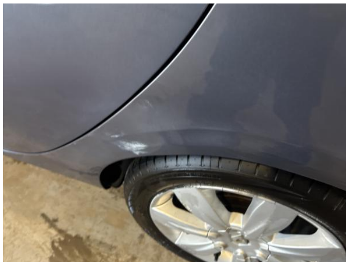
10: Qtr Panel nsr Dented With Paint Damage
