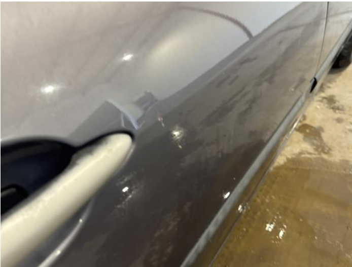
17: Door osr Dented With Paint Damage
