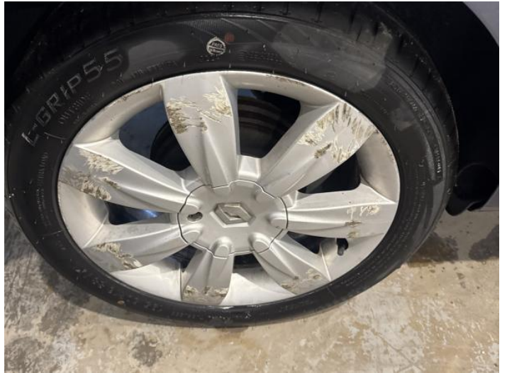
16: Wheel osr Scratched Over 50mm
