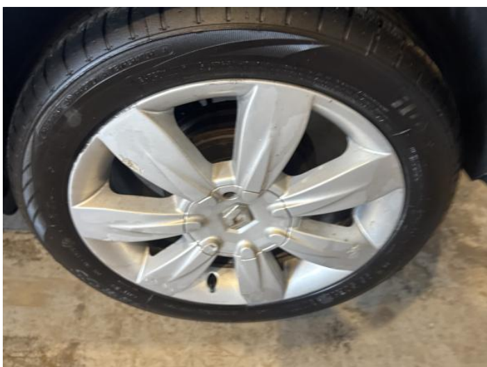
11: Wheel nsr Scratched Over 50mm
