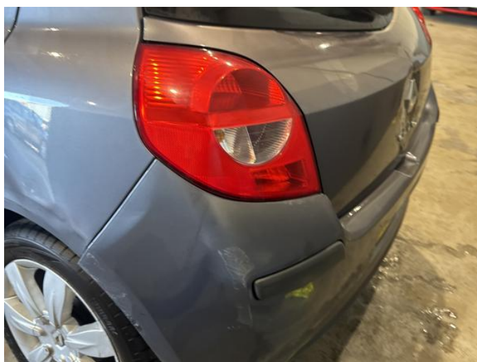
12: Bumper Rear Poor Previous Repair Poor Paint
