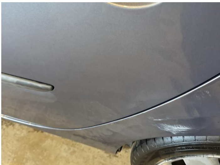
9: Door nsr Dented Over 30mm
