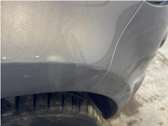
21: Wing osf Scratched UpTo 25mm Thru Paint
