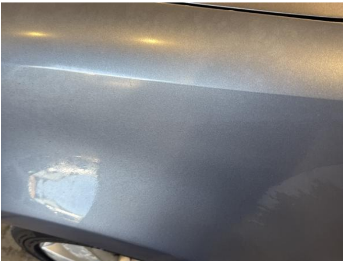
5: Wing nsf Poor Previous Repair Poor Paint
