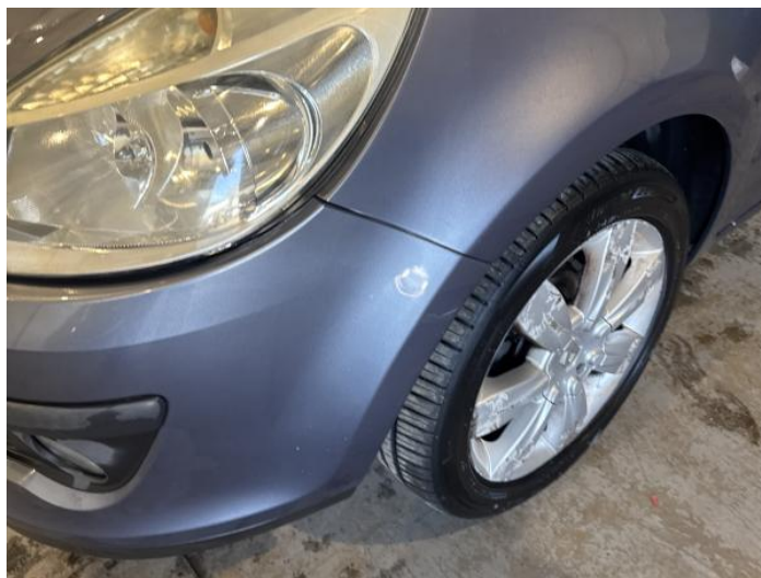
2: Bumper Front Scratched 25 to 100mm Thru Paint
