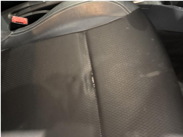
24: Seat Base Cover osf Torn UpTo 3mm
