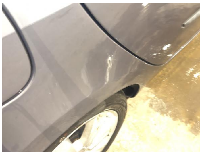
14: Qtr Panel osr Dented Between 10mm + 30mm
