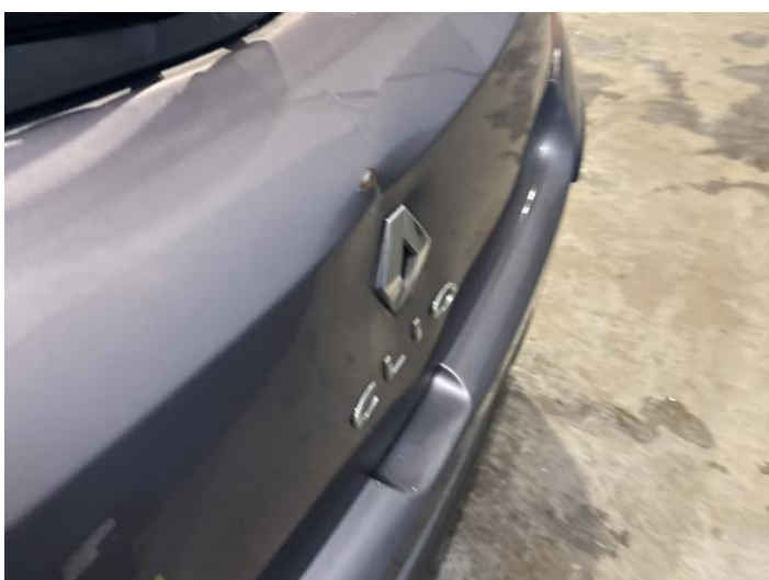
13: Boot Lid Dented With Paint Damage
